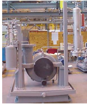
Figure 8: Small and large OH2 pumps with auxiliaries mounted in front of the suction nozzle area
