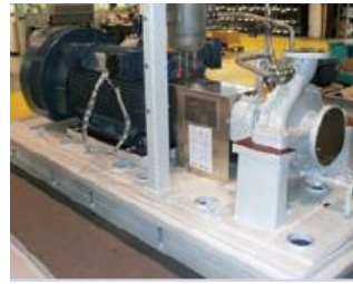
Figure 4: Flat deck type with a mounted sloped gutter drain and extending beneath the pump and driver
