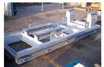
Figure 7: Open deck of the three basic designs with no deck/top plate (grouted or non-grouted)
