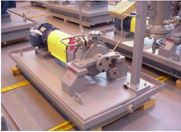
Figure 8: Small and large OH2 pumps with auxiliaries mounted in front of the suction nozzle area
