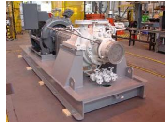
Figure 5: Sloped deck plate between the side rails and extending beneath the pump and driver
