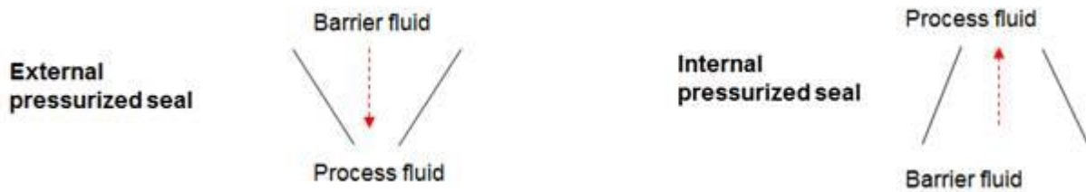
Figure 9: Tendency of seal gap geometry for an external (left) and internal (right) pressurized seal. The red arrow indicates the leakage path (leakage from high pressure barrier fluid towards lower pressure process fluid).
