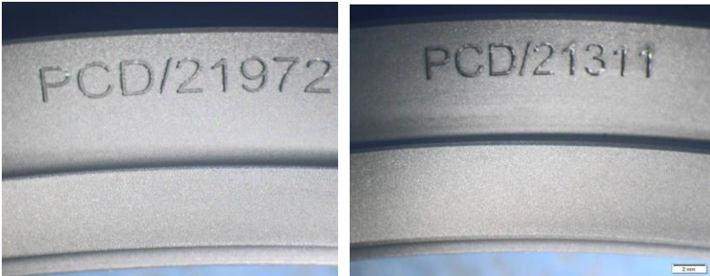
Figure 14: Seal face (left) and seat (right) inspection after the performance test
