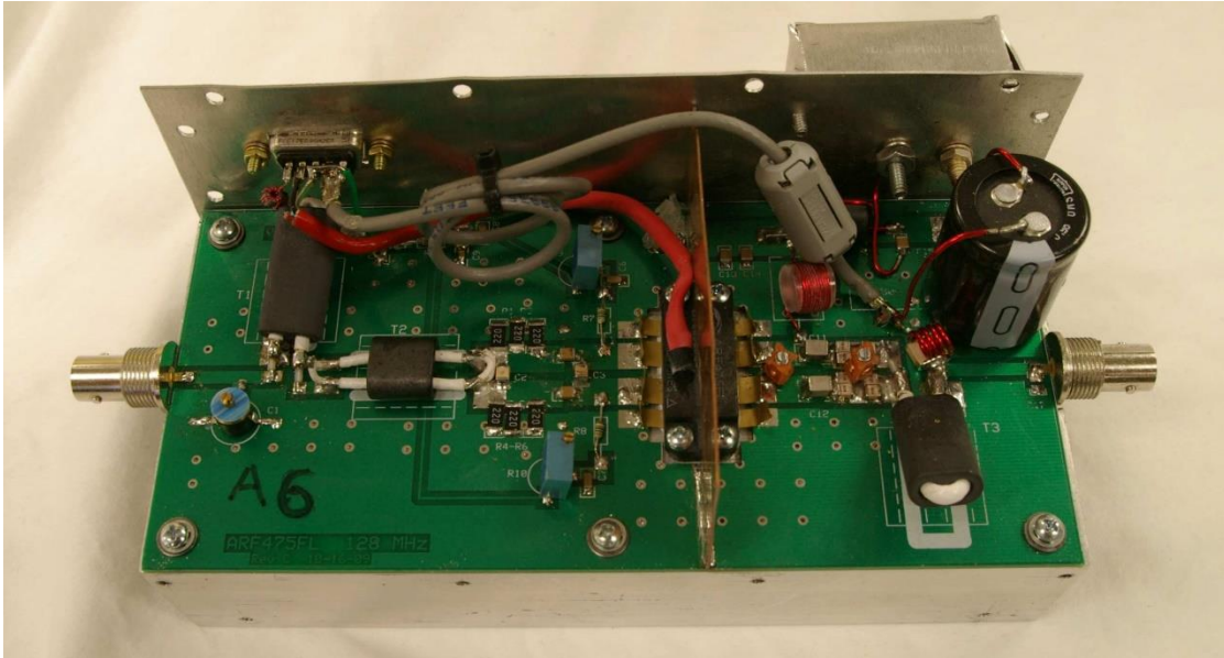
Figure 4.15: An LOI amplifier module based on the ARF475FL. Input on left, output on right. This module include a thermal sensor on the MOSFET package, and a biasing network to switch the PIN diode TR switch.
