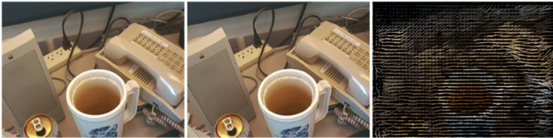
Figure 2.12: Litwinowicz's technique for obtaining impressionist effects. Two frames and the optical flow field that maps pixels from one frame to another
