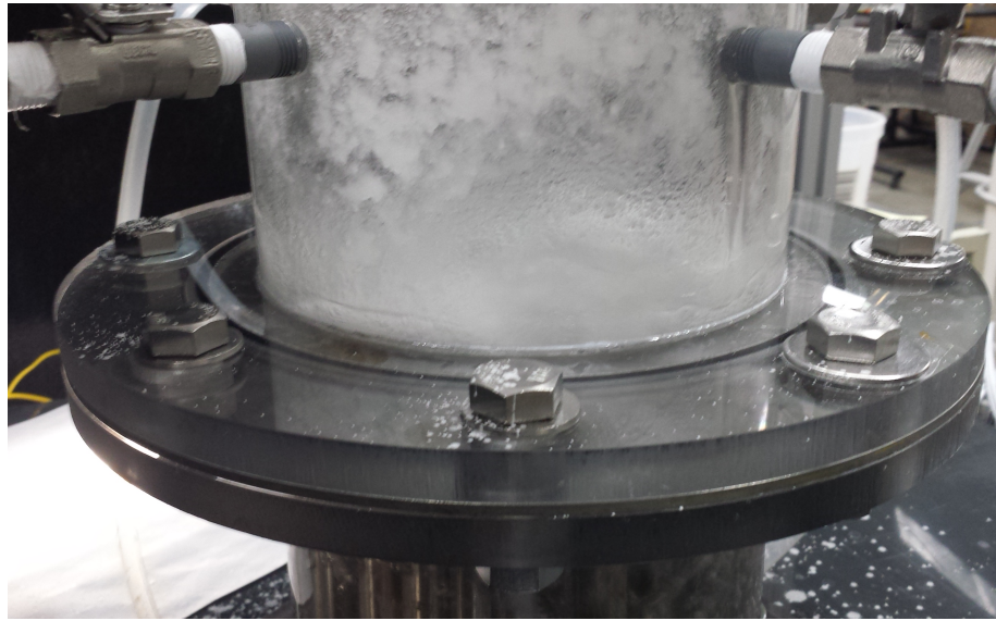
Figure 6.2: Boric acid precipitate at top of test section during experimental runs near termination.
