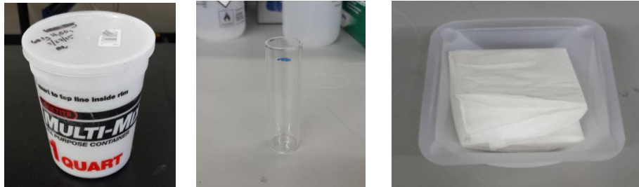
Figure 1a. Plastic container used for boric acid preparation. b. Glass vial for sampling with 16 mL indicator. c. Tray and foils used for sample drying.
