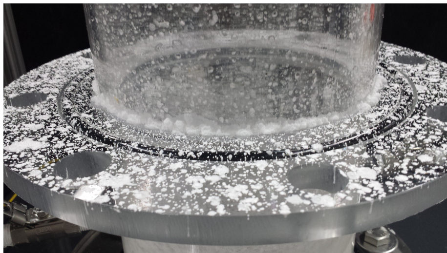
Figure 6.3: Boric acid precipitate deposition during unlidded experimental runs.
