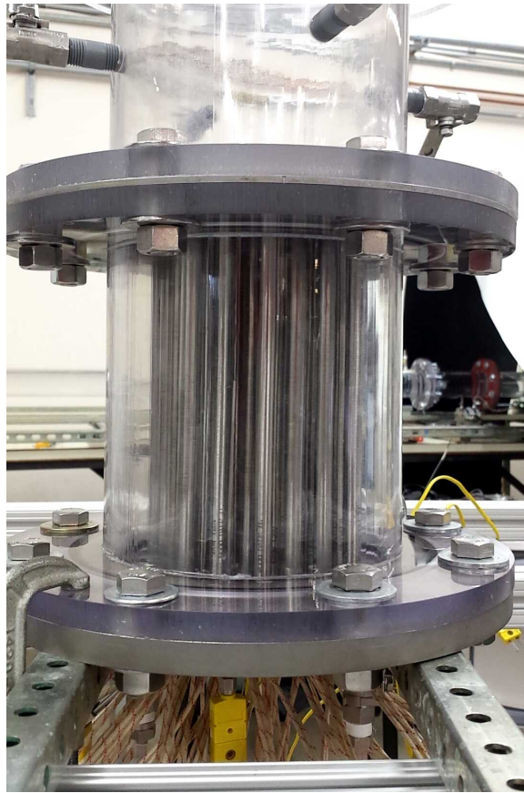
Figure 2.1: The fully assembled PASTA facility test section.
