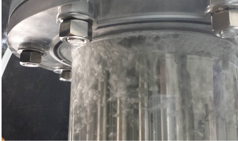
Figure 6.1: Volatile boiling in test section during experimentation.
