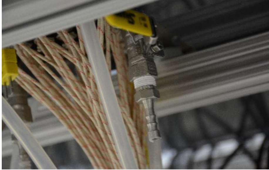
Figure 2.4: Photo of the valved ports at the bottommost flange of the PASTA facility test section.
