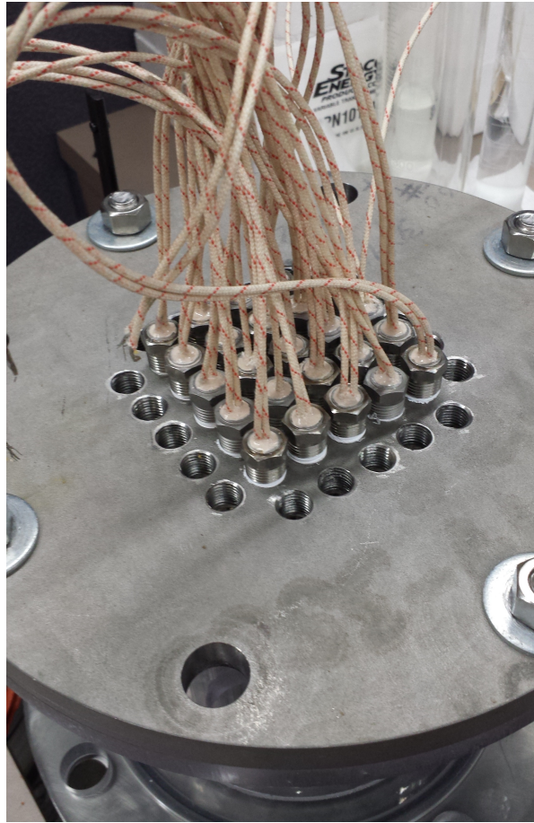
Figure 2.3: Bottom plate flange with shown threaded holes to secure heating rods at bottom of test section.
