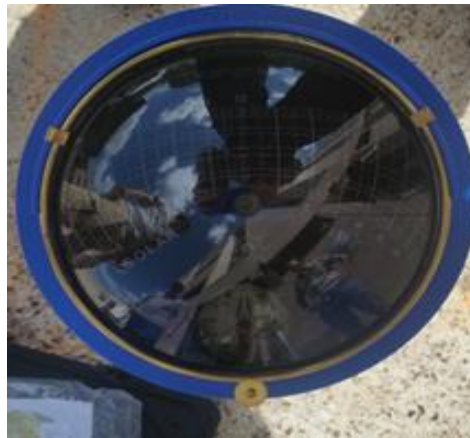
Fig. 1.20 Solar site assessment for LOCATION 1 using Panorama SPF chart
