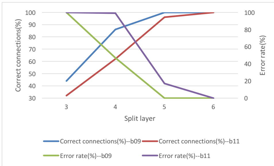
Figure 15: Correct connection rate and error rate vs. split layer for “Physical attack” on circuits b09 and b11
