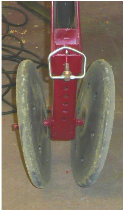
Figure 7- Original Press Wheel Construction.
