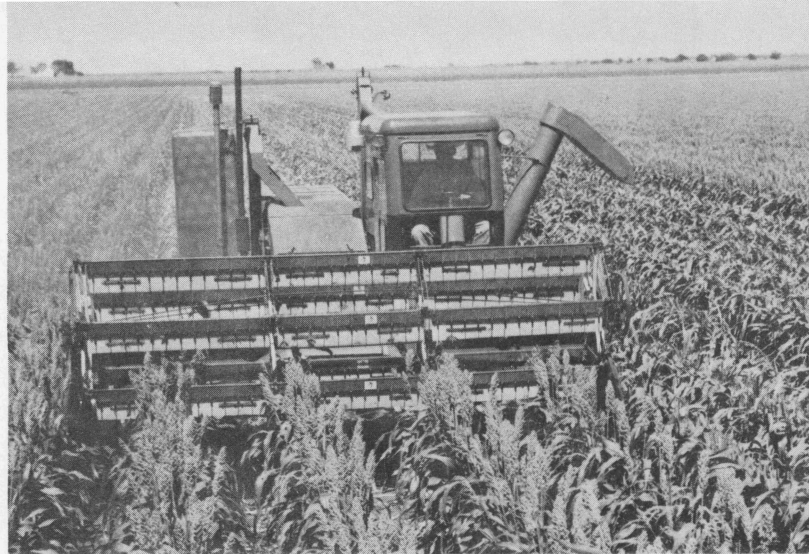
Figure 14. Combines should be adjusted carefully to keep cracked kernels and trash in the threshed grain to a minimum. This will help avoid insect and heating problems in storage.
