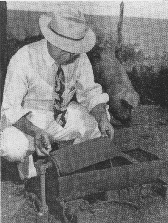
Water Trough Made Out of Oil Field Pipe (Note partition between float valve and drinking place)
