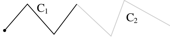
Figure 4.3: The reachable volume of a chain that is composed of two smaller chains C_1 (black) and C_2 (gray) is the Minkowski sum of the reachable volumes of C_1 and C_2 .
