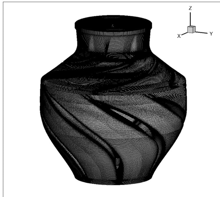
Figure IV-9: Illustration of the mesh of the whole stage
