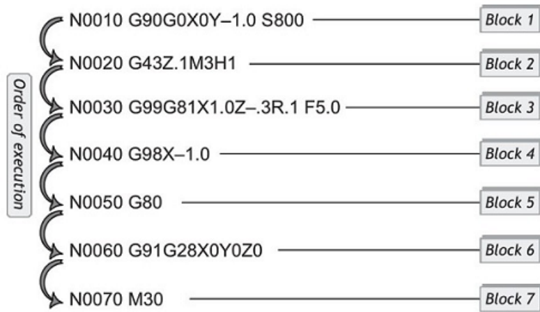
Figure 1.7: The execution sequence of a part program [18]
