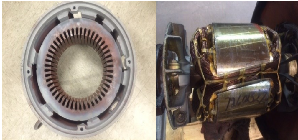
Figure 2.1. Synchronous generator stator and rotor.
