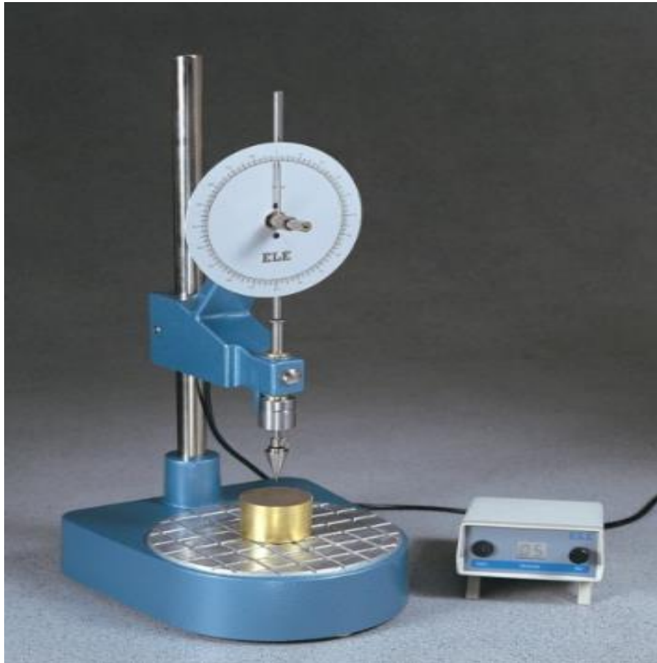
Figure 25 Typical fall cone penetrometer, (After ELE International).
