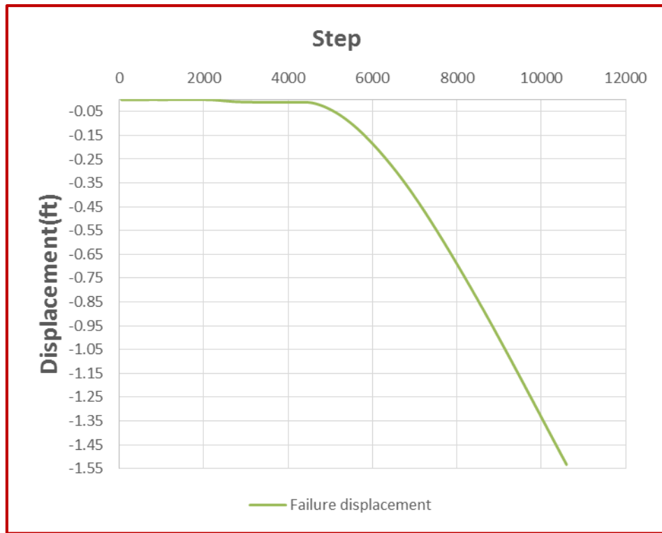
Figure 78 Horizontal deformation at depth of 12 ft after the second stage of construction.
