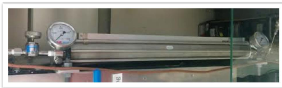
Figure 6. Piston sampler for pressurization of gas samples
