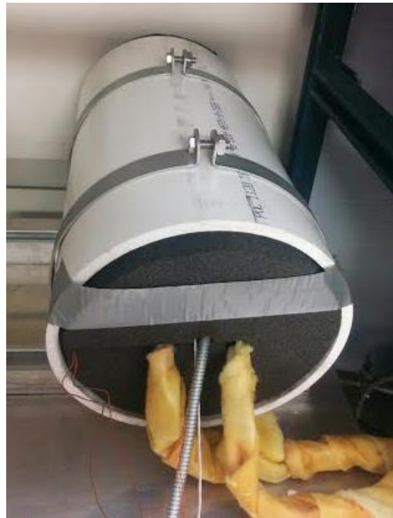
Figure 8. FOAMGLAS insulation inside a PVC cylinder and secured with metallic clamps
