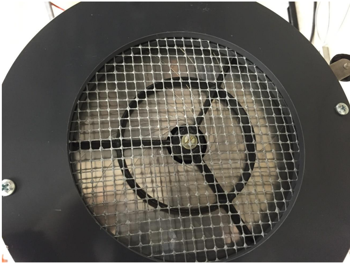
Figure 10. Close-up picture of the iris damper in the 2.5% open position
