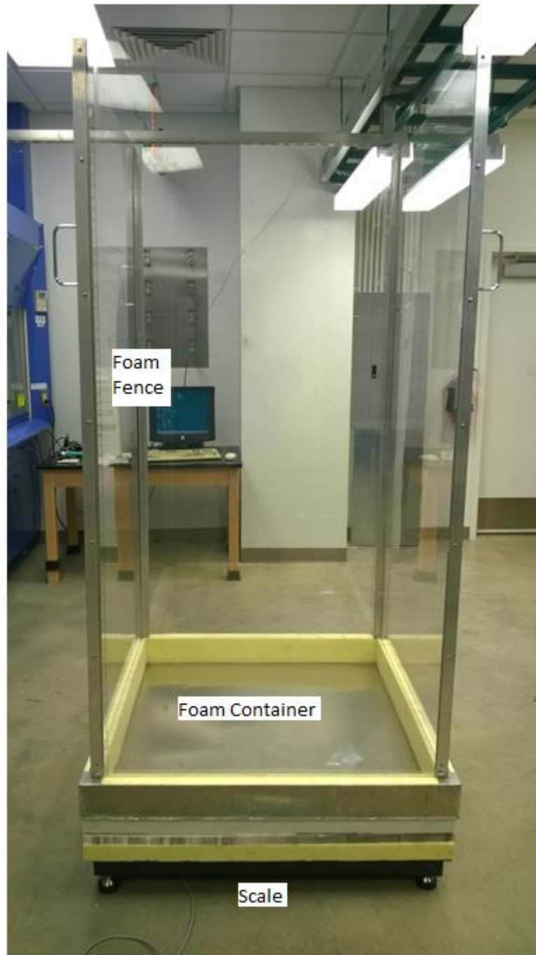
Figure 12. Picture of the foam container and fence showing the scale located beneath it to measure the mass
