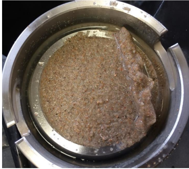
Fig. 14 - Ceramic disc during scrape process.
