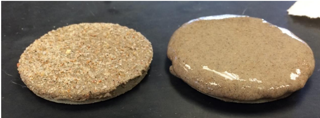
Fig. 16 - Comparison of scrape (left) and base (right) tests shows the scraping, which replicates stabilizers, yields a superior filter cake. This results in a better API FL and thus a reduction in wellbore enlargement.
