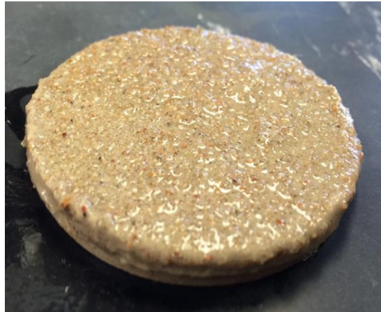
Fig. 9 - Ceramic disc after optimal bridging test.
