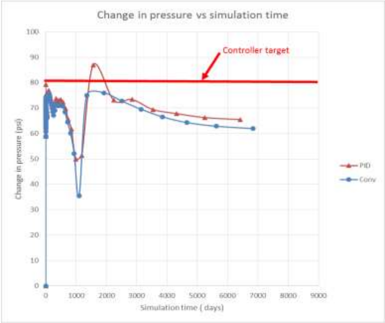
Figure 15: Pressure change versus simulation time (base case with pressure limiting factor)
