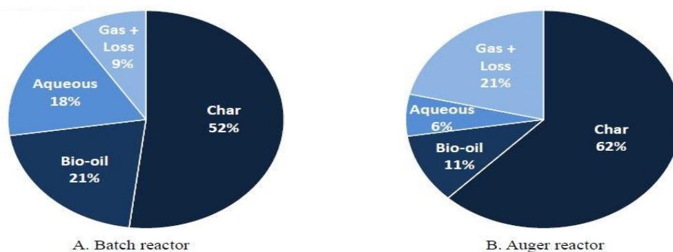
Figure 2. Mass product yields from each reactor at 500°C.
