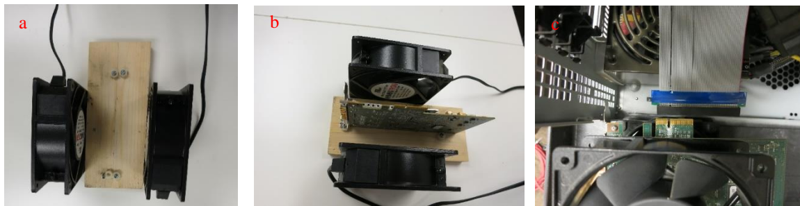
Figure 8: a) The cooling solution without digitizer card installed. b) The cooling solution with digitizer card installed. c) The digitizer card being plugged into the PCI-e bus extender.
