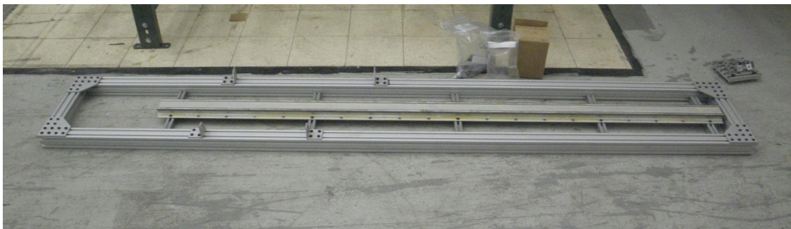
Figure 45. Lower camera rack frame with precision sliding track.
