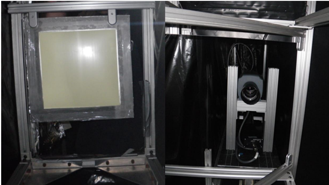
Figure 48. Images of the NIS1 with the scintillator and holder (left) and the camera and sled (right).
