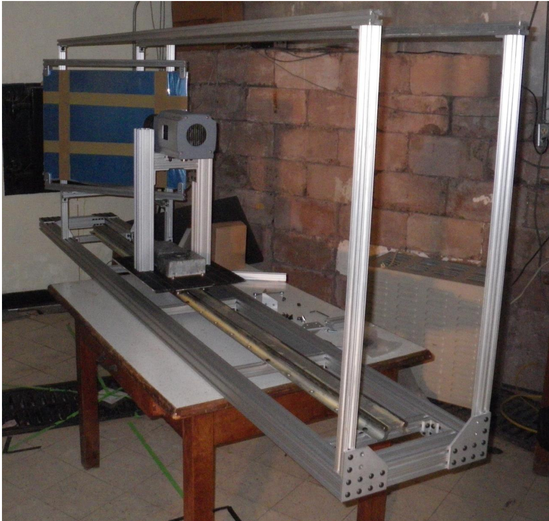
Figure 46. Assembled camera rack with front surface mirror mount and camera sled.
