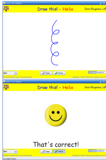
Figure 2.5: The application includes a sketch-recognizer that can determine children’s drawing correctness: (top) the application asks children to draw simple shapes with text, and children can draw the shapes on the sketch-panel and (bottom) after children draw the shape, the application determines the correctness of the shapes [173].
