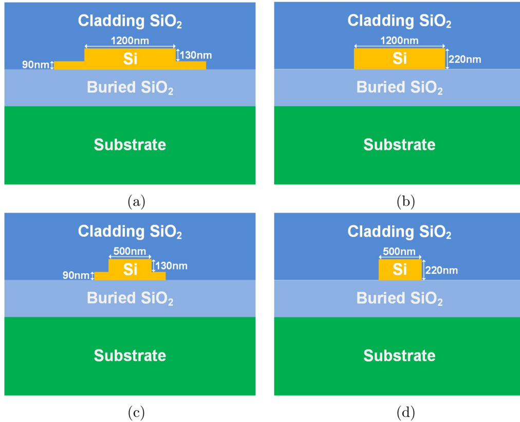
Figure 2.7: Cross section views of (a) multi-mode rib waveguides, (b) multi-mode strip waveguides, (c) single-mode rib waveguides and (d) single-mode strip waveguides.
