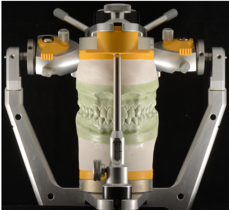
Figure 1. Mounted Casts On SAM 3 Semi-Adjustable Articulator
