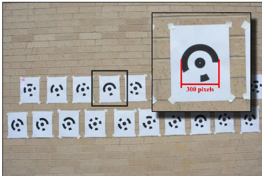
Figure 2-8. Photo of coded targets shown in a maximum recommended size. Photo was taken by a camera with APS-C sensor (with 18 mm Focal Length and 2.0 m away from the CTs) (6000 x 4000 pixels / 300dpi). The targets (20.0 mm center point radius) have 300 pixels at the outer circle. 300 pixel diameter is a recommended maximum size for coded targets. (Photo: Yamafune)
