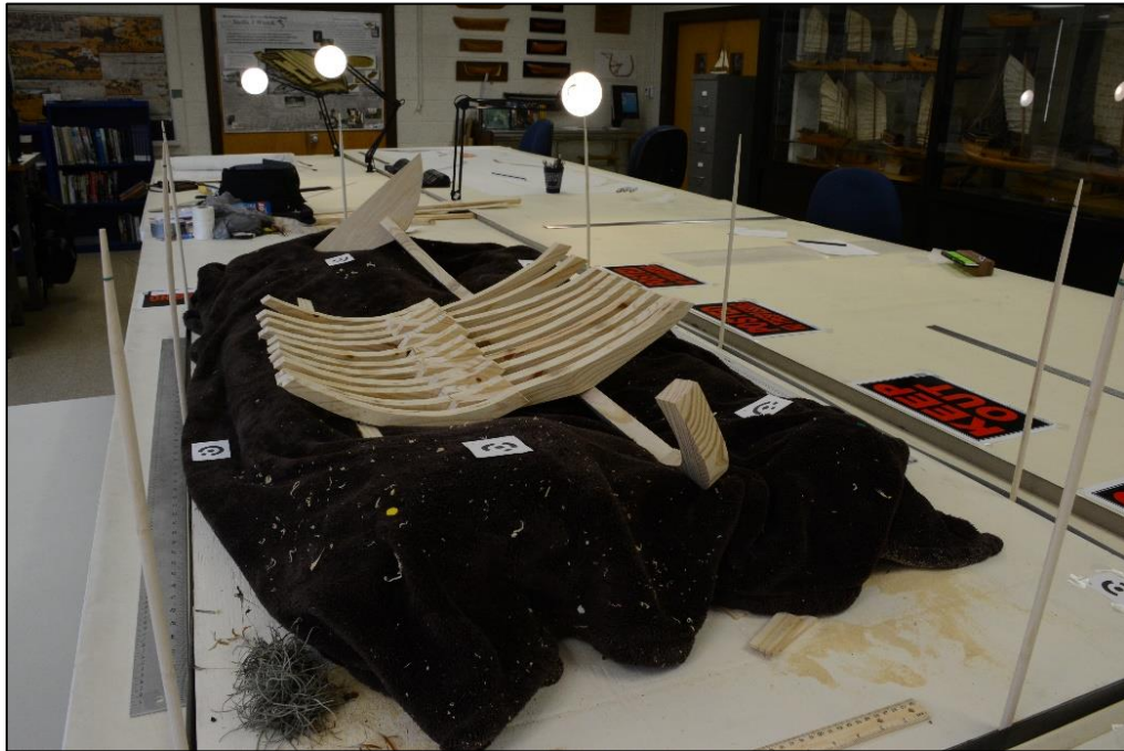
Figure 3-31. An example of photos of the saveiro wooden model that were disabled for Build Dense Cloud process. The photo was taken obliquely; therefore it displayed sides of frames as if there were surfaces between frames. (Photo: Yamafune)
