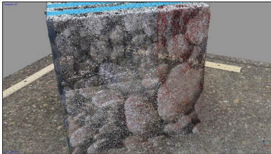
Figure 3-8. Accuracy: Low setting on Build Dense Cloud process. Total number of the points is 2,573,953. (Image: Yamafune)
