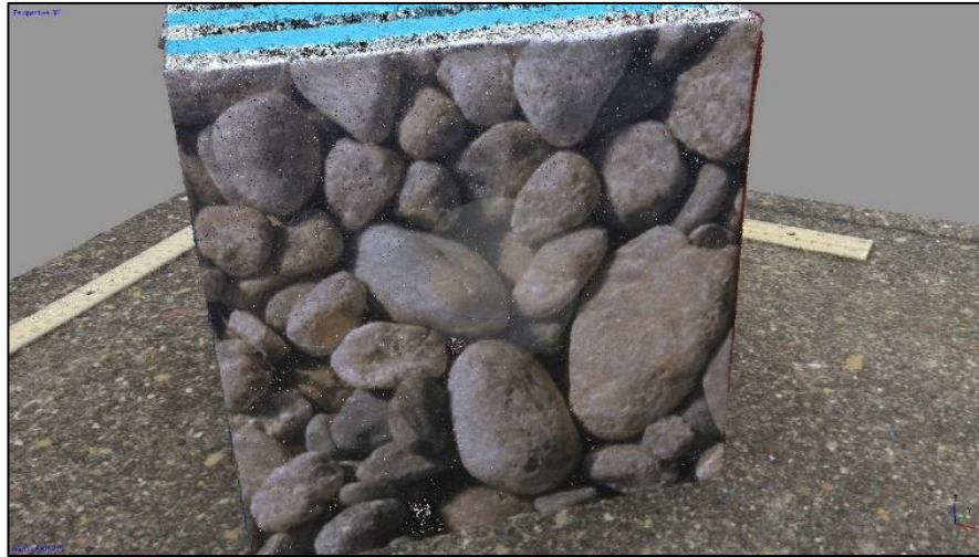
Figure 3-7. Accuracy: Medium setting on Build Dense Cloud process. Total number of the points is 9,979,748. (Image: Yamafune)
