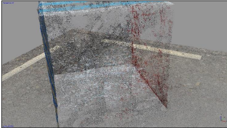
Figure 3-9. Accuracy: Lowest setting on Build Dense Cloud process. Total number of the points is 644,590. (Image: Yamafune)
