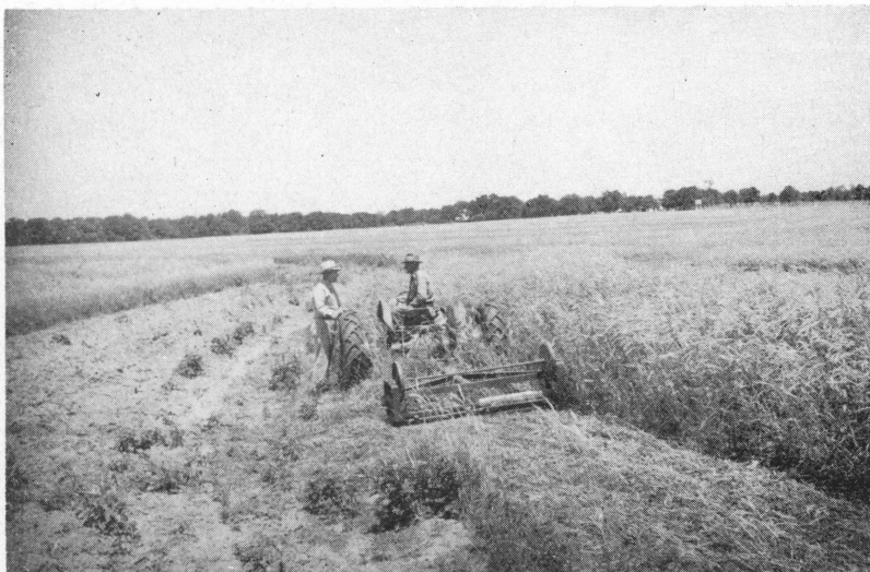
Working vetch and winter grain into the soil for green manure with the use of a stalk cutter followed by a tandem disk.
