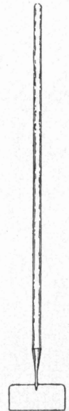
Silage cutter to get silage out that has been put in the trench uncut.
