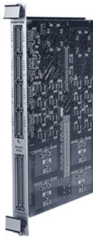
Fig. 3-17 A photograph of the I/O board Pentek 6102 [85].
