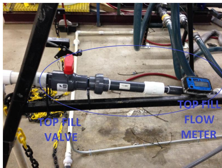
Fig. 59 – Top Fill Line Configuration
