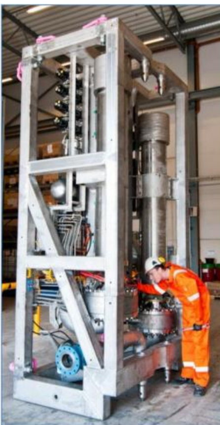
Fig. 3—EC-Drill™ Subsea Pump Module (Mirrajabi et al. 2012)
