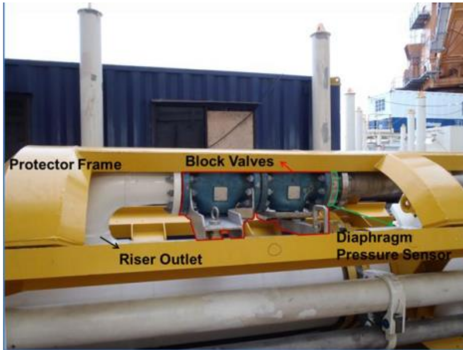
Fig. 4—EC-Drill™ Modified Riser Joint (Mirrajabi et al. 2012)
