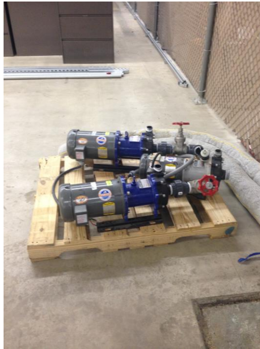
Fig. 13—Scaled Pumps for Riser Simulator
