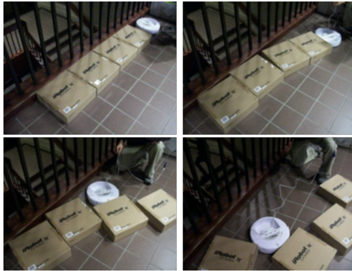
Figure 4.3: Square object detaching progress by repetitive prying motions.
