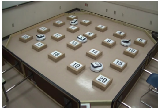
Figure 3.4: An example of object clustering scenario: 20 square objects (brown boxes) and 5 robots (white round devices).
