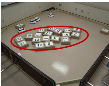
Figure 5.1: An example of an asymmetric cluster in an experiment. The cluster is elliptical in shape (see red oval).
