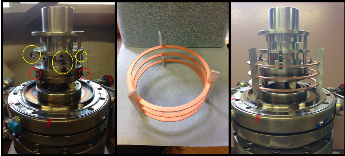
Figure A.4: Ion source lens elements and accelerator column simulation jig. Left) Yellow circles indicate focus electrode “fingers”, whereas red circles indicate the equivalent component locations on the extractor electrode (missing “finger” on left has since been replaced). Center) Jig created to simulate the inner ring contact points of the accelerator column, allowing lens element “fingers” to be shaped appropriately before blind assembly. Right) Jig mounted on ion source to test the configuration of contact “fingers”.
