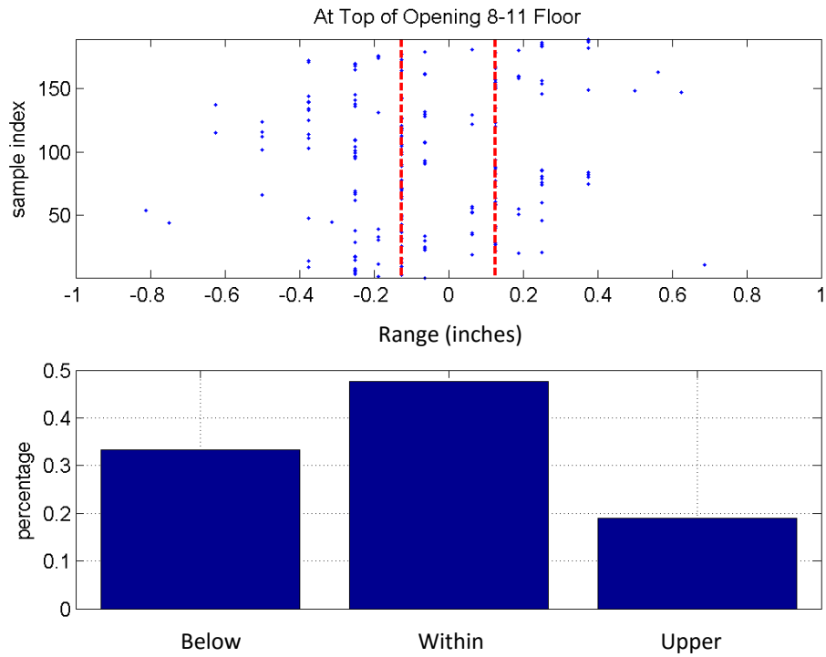
Figure 49. Plot of tolerance results at the top of the openings, from 8 th to 11 th floors.
