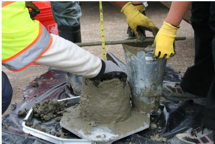
Figure B.28. Slump Measurement (CC).
