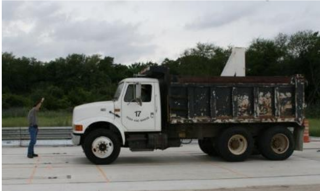
Figure 5.16. Static Loading with Dump Truck.
