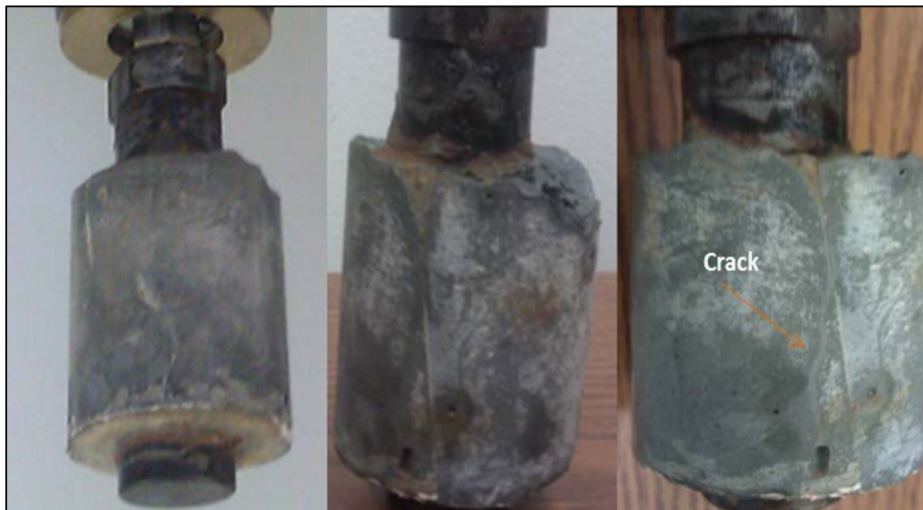
Figure 19. Cyclical loading caused a radial crack in sample II-A.
