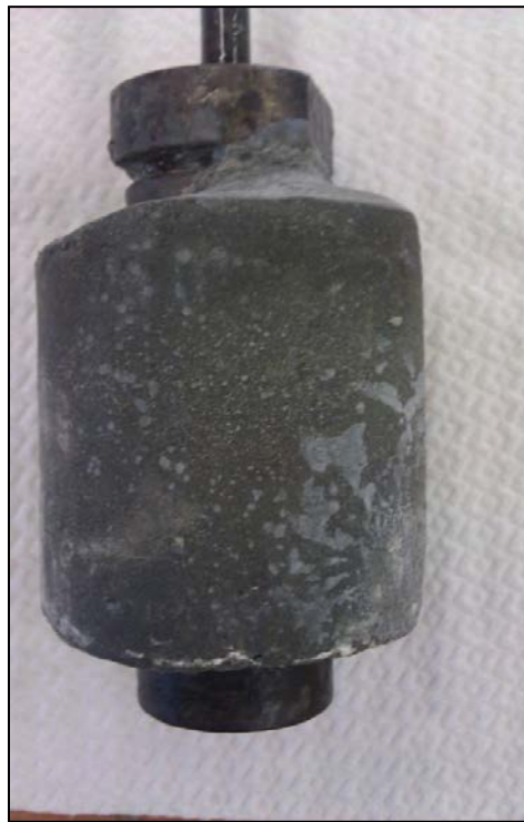
Figure 41. Sample IV-E, No crack after 8 cycles, repeatability test.
