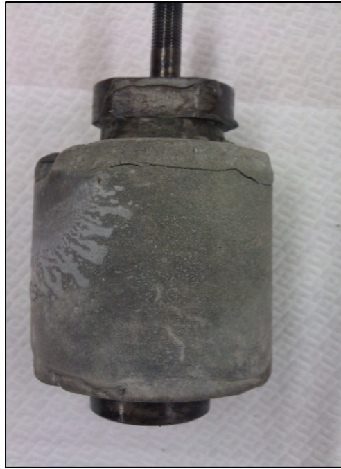
Figure 35. Sample I-F, a micro crack.
