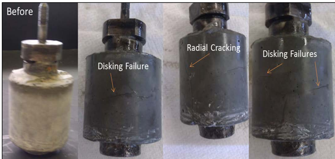
Figure 24. Sample I-B, radial cracking and disking, cement failures after 106 cycles.
