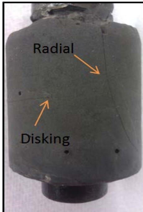
Figure 38. Sample II-F, cracked after 13 cycles.
