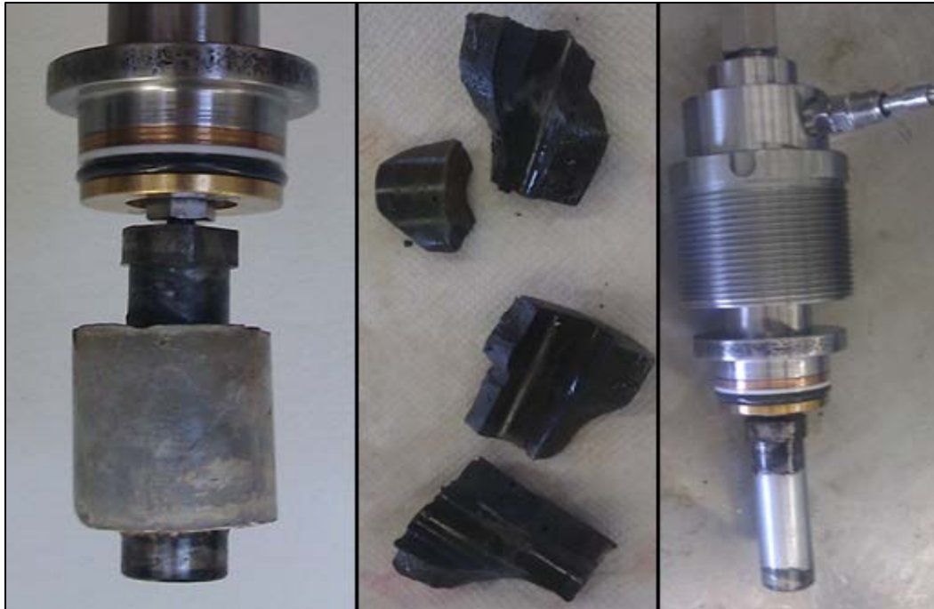
Figure 17. Inconsistent confining pressure caused severe cement sheath destruction.
