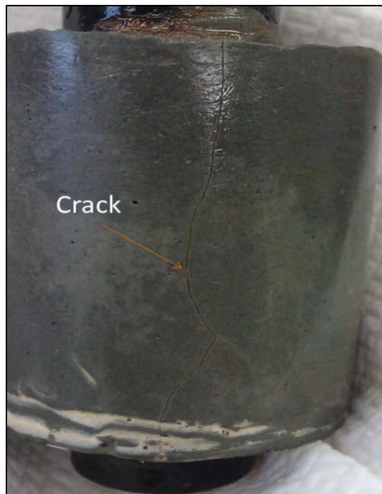
Figure 21. One radial crack in sample III-A after the test.
