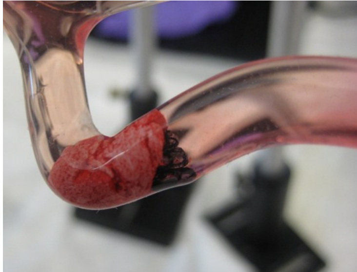
Figure 3.1. Flower-shaped thrombectomy device off-centered after actuation. Device was painted with a black marker for better visualization.
