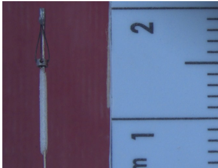
Figure A1. First prototype of the SMP-SMA thrombectomy device made assembled with the nitinol wire-based MNF and crimped SMP foam.
