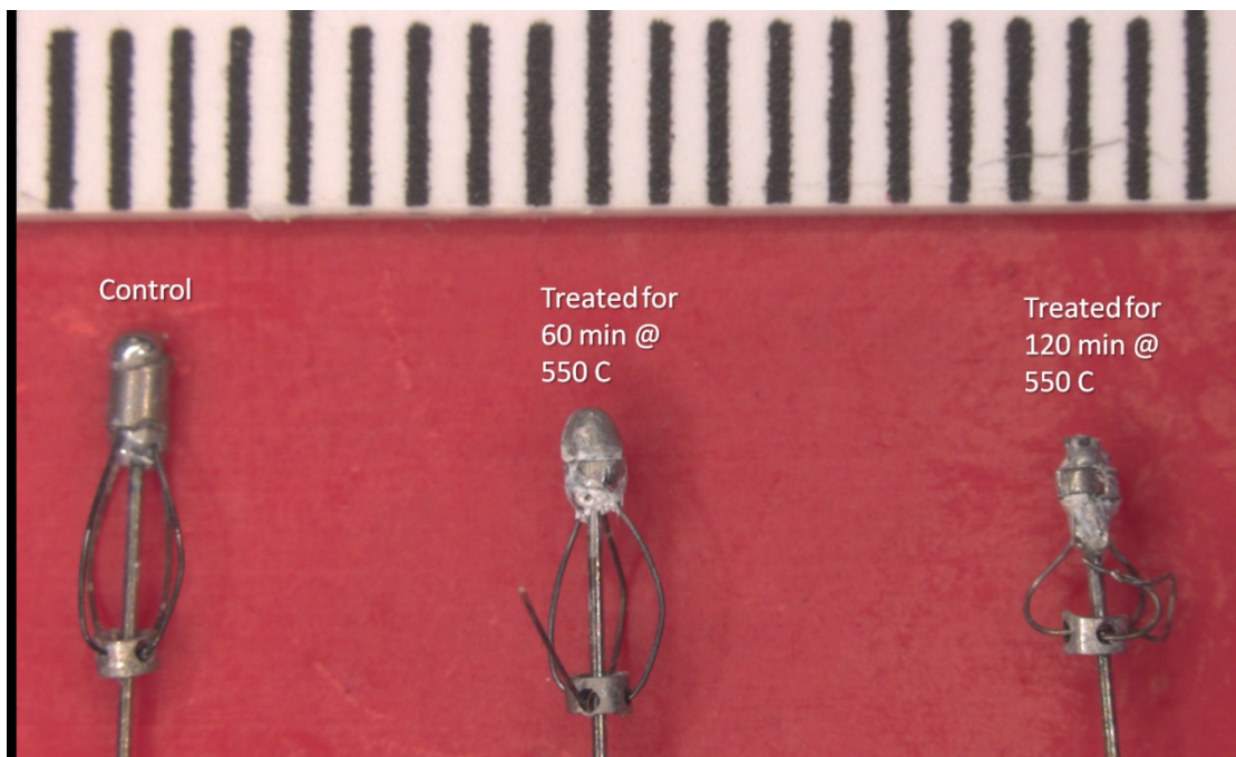
Figure A4. MNFs assembled with control wire and heat treated wire at 550 °C for 60 and 120 min before (a) and after (b) axial compression.
