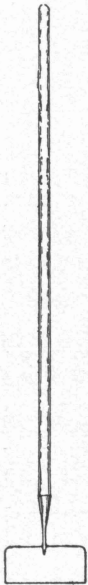
Silage cutter to get silage out that has been put in the trench uncut.
