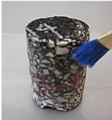
Figure 11: Application of epoxy
