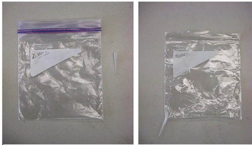
Figure 12: The piping tool used for epoxy. Pre-assembled (left) and assembled (right).
