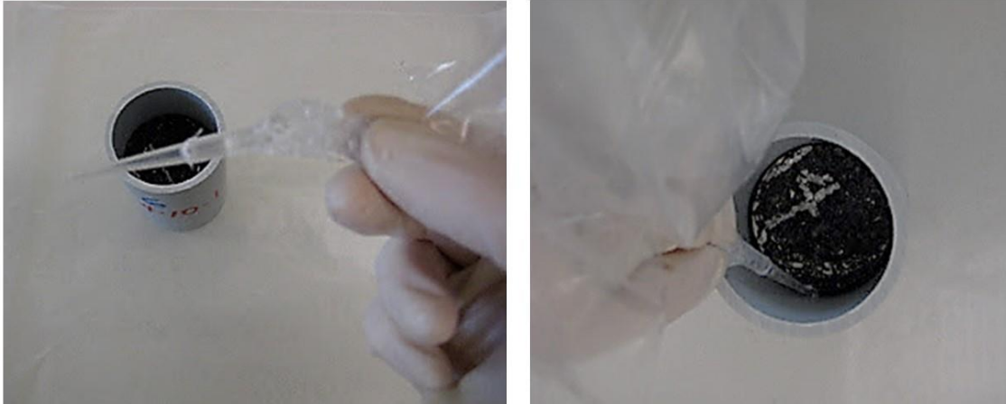
Figure 13: The piping tool with epoxy (left) and in use (right)
