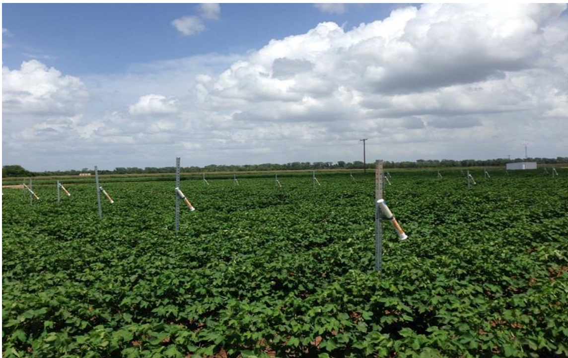
Figure 2.1. Smartcrop™ infrared sensors were installed on a 2 m perforated pole about half-way into each plot, on the third row, pointing southeast. Brackets mounted on the pole maintained sensors at a fixed 45° angle from the soil surface throughout the season. Constant adjustments in height were made to maintain sensors about 20-30 cm above the crop canopy, which resulted in an approximate 0.5 m 2 field of view.
