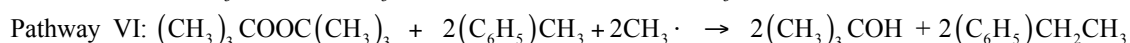
Figure 18. Possible identified pathways for the decomposition of DTBP in toluene. Adapted from AlDeeb [119]
