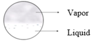
Figure 29. Schematic of a circular exit point wherein there is two-phase flow.
