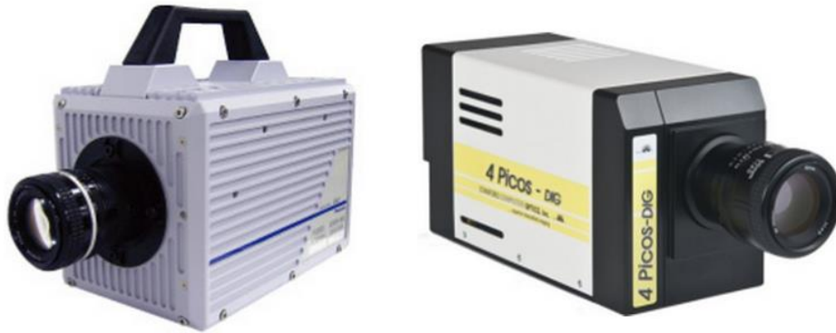
Figure 14. CMOS (Copyright © Photron FASTCAM SA5) and ICCD (Copyright © Stanford Computer Optics) High Speed Camera [49]
