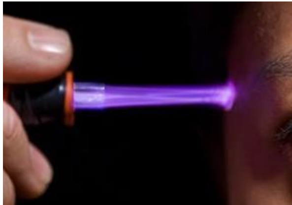
Figure 4. Dielectric Barrier Discharge (DBD) on Person's Forehead [23] (Copyright © PEDL TAMU)
