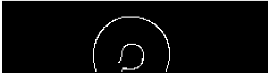
Figure 65. Boundary Identification Using “canny” Algorithm
