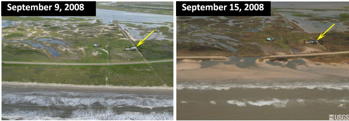
Figure 1.6: Damage to east end of Follett's Island from Hurricane Ike [7]. Arrow indicates reference point for comparing pre- and post-storm images.
