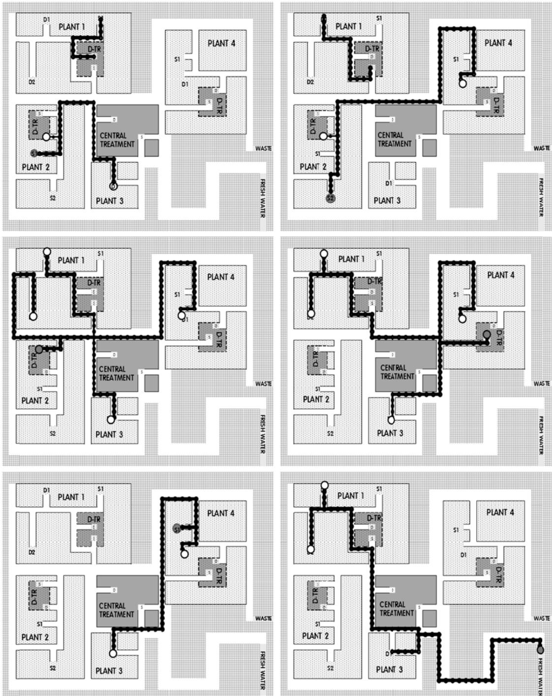
Figure 36. Forward pipeline branching with 90° pipe bending illustrated (Case 1)
