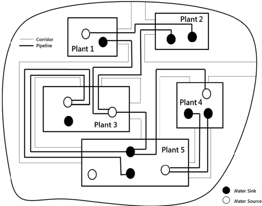
Figure 20. Typical output of a source-sink mapping activity, for the design of interplant water networks
