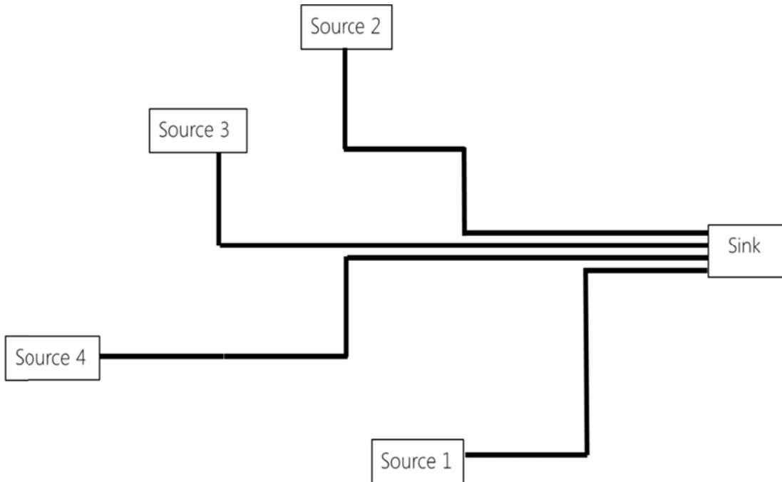
Figure 22. An unmerged pipeline connectivity demonstration for a given water sink, receiving water from several nearby water sources
