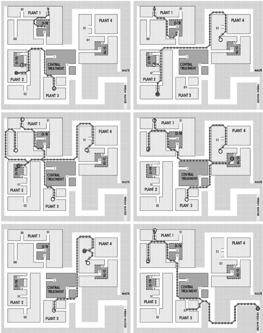
Figure 37. Forward pipeline branching with  $90^{\circ}$ ,  $45^{\circ}$  and  $135^{\circ}$  pipe bending illustrated (Case 2)
