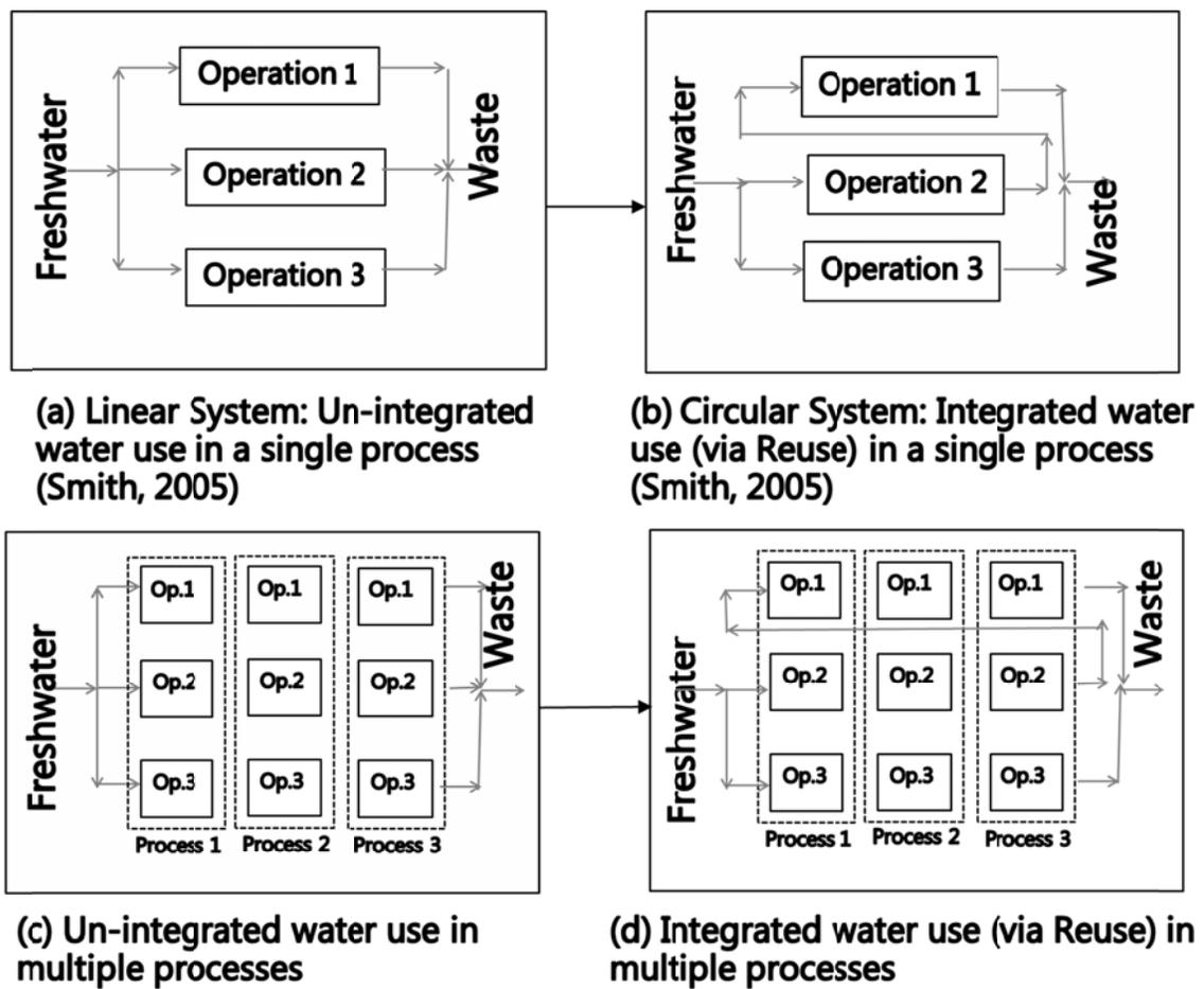
Figure 1. Water re-use concept on a local vs. global level
