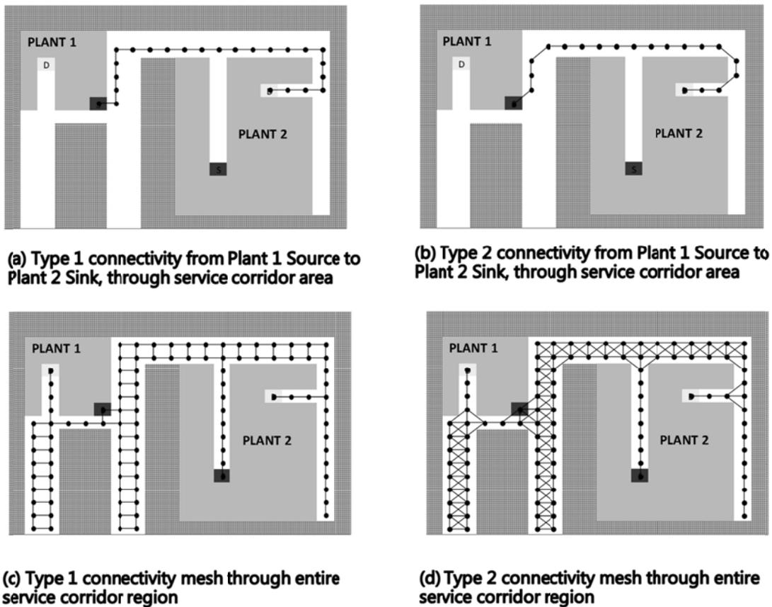
Figure 5. Piping Connectivity illustrated for Figure 3's Small-Scale Illustration
