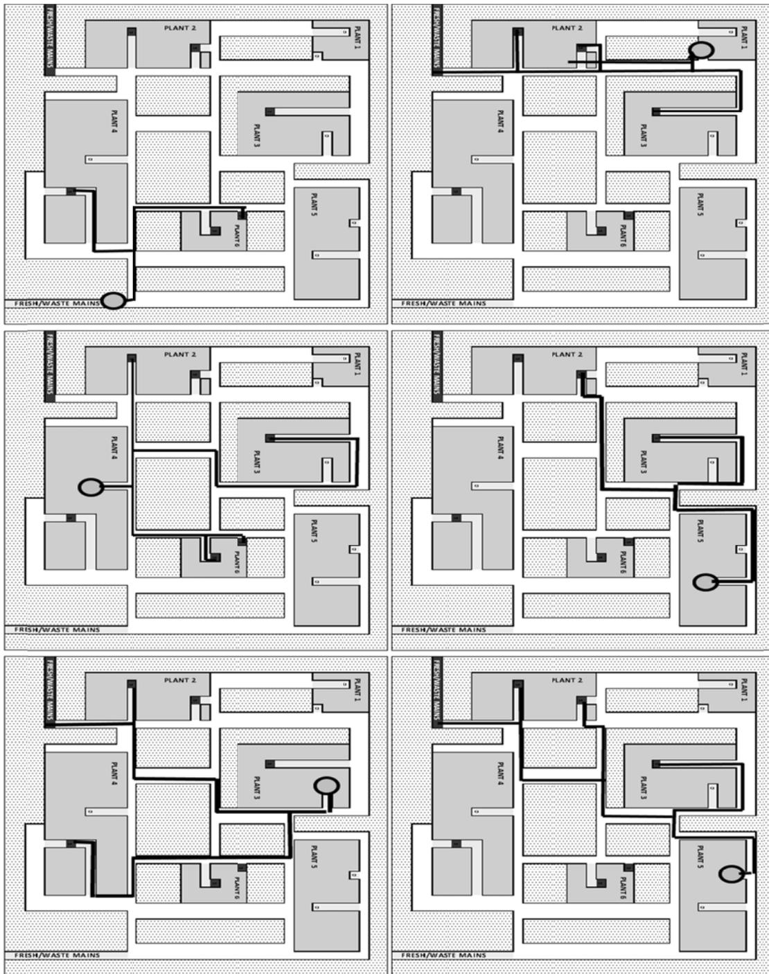
Figure 34. Case 4 interplant piping illustrated after merging, via backward branching
