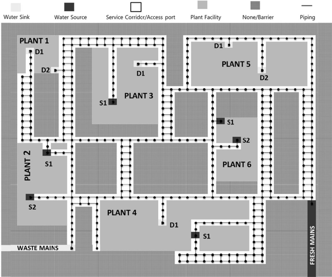
Figure 6. Industrial City Case Study Layout, with Type 1 connectivity mesh illustrated
