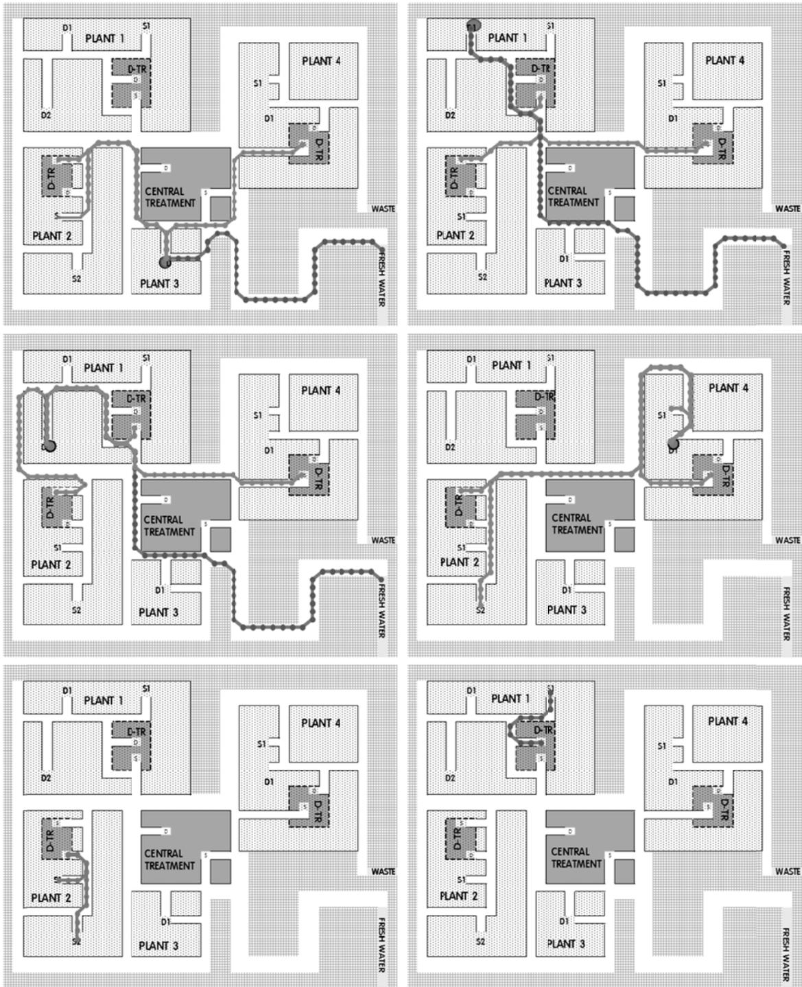
Figure 39. Backward pipeline branching with  $90^\circ$ ,  $45^\circ$  and  $135^\circ$  pipe bending illustrated (Case 4)
