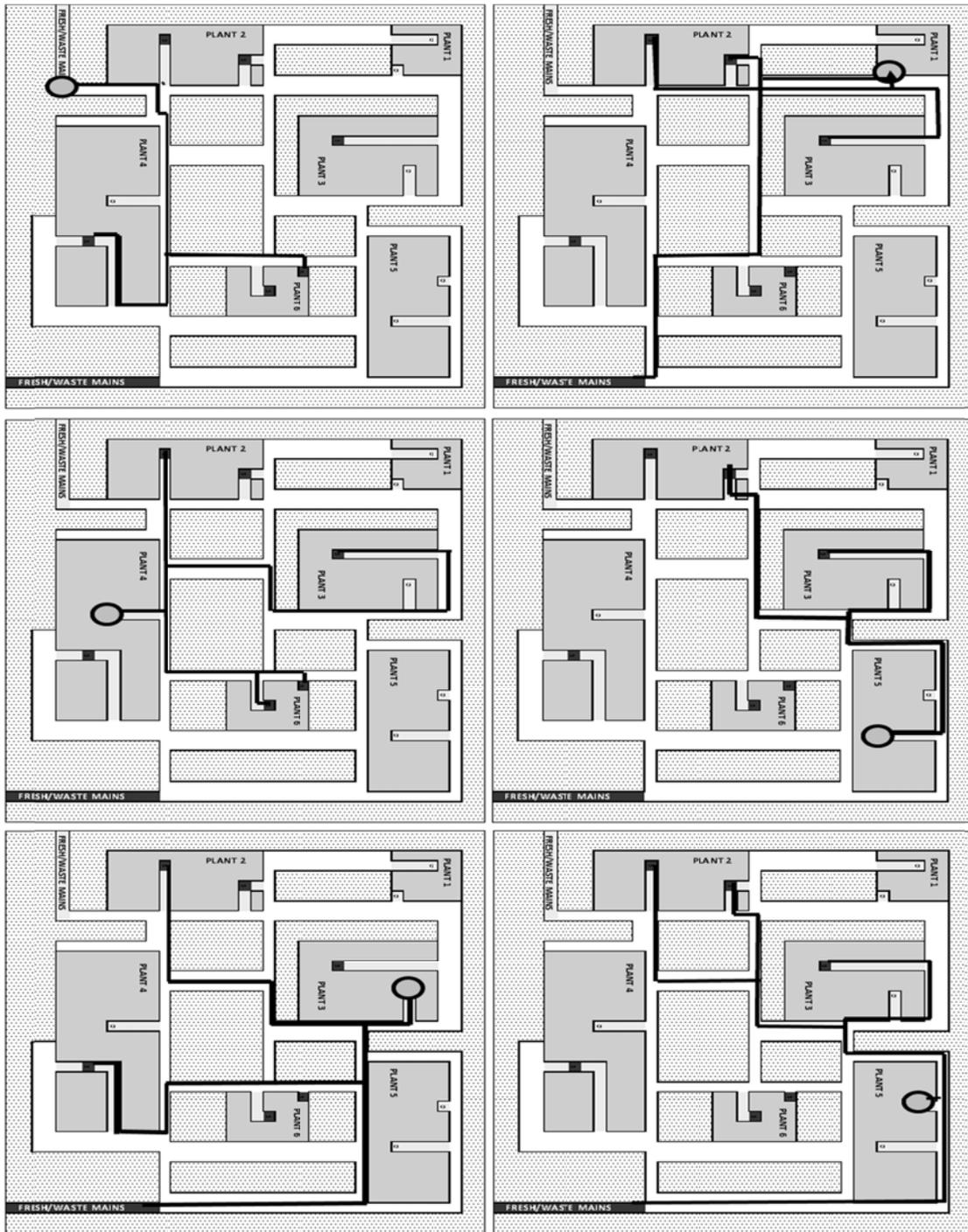
Figure 33. Case 3 interplant piping illustrated after merging, via backward branching
