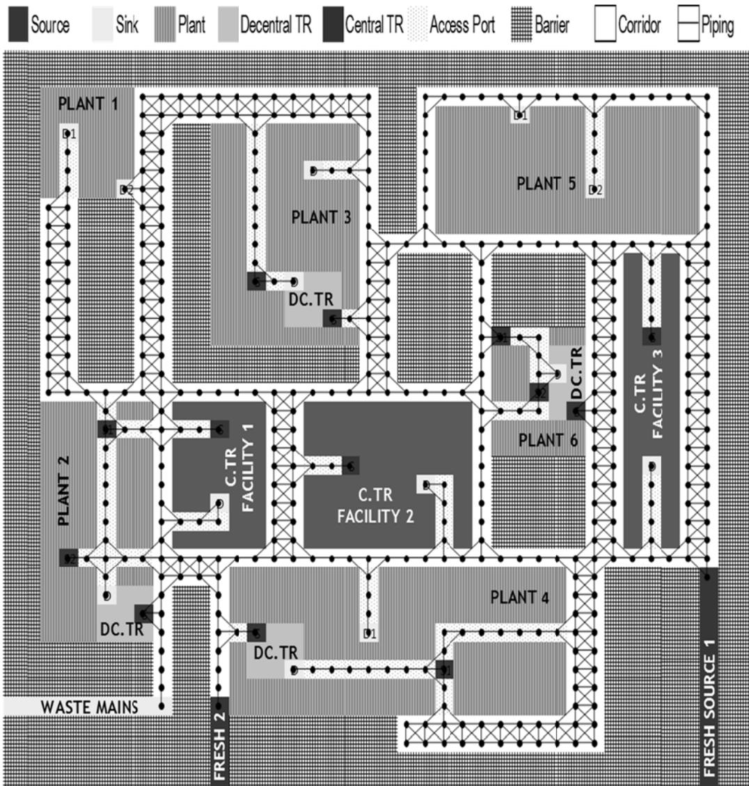
Figure 14. Industrial City Layout, with Type 1 connectivity mesh illustrated
