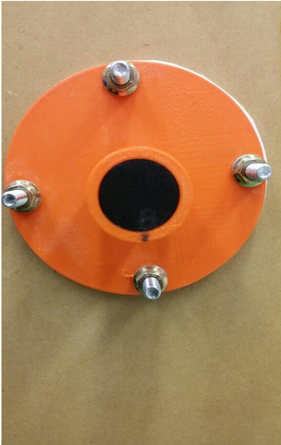
Figure 35. Plug attached to the pipe assembly
