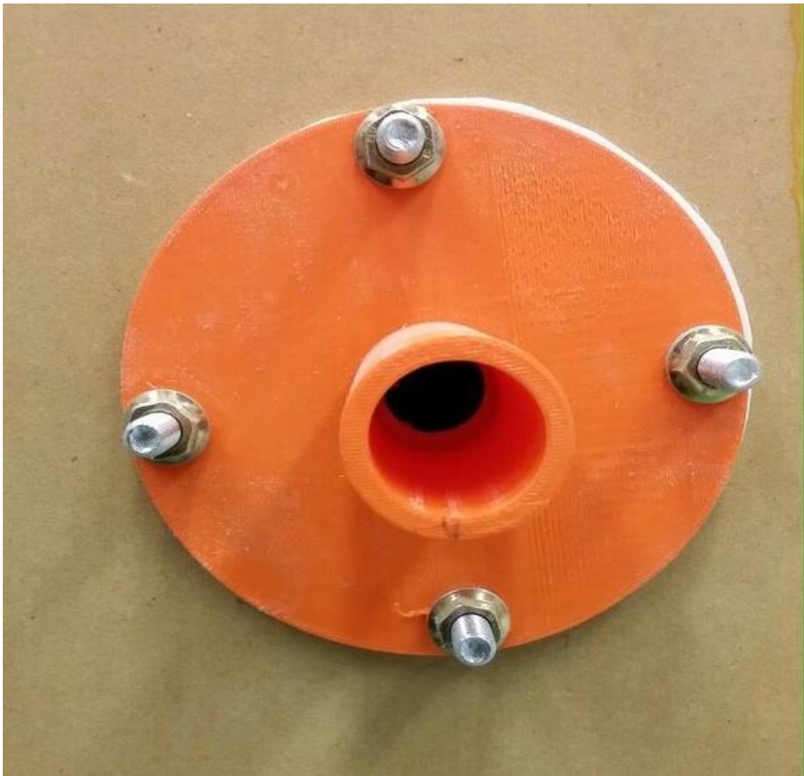
Figure 34. Pipe assembly attached to the test box
