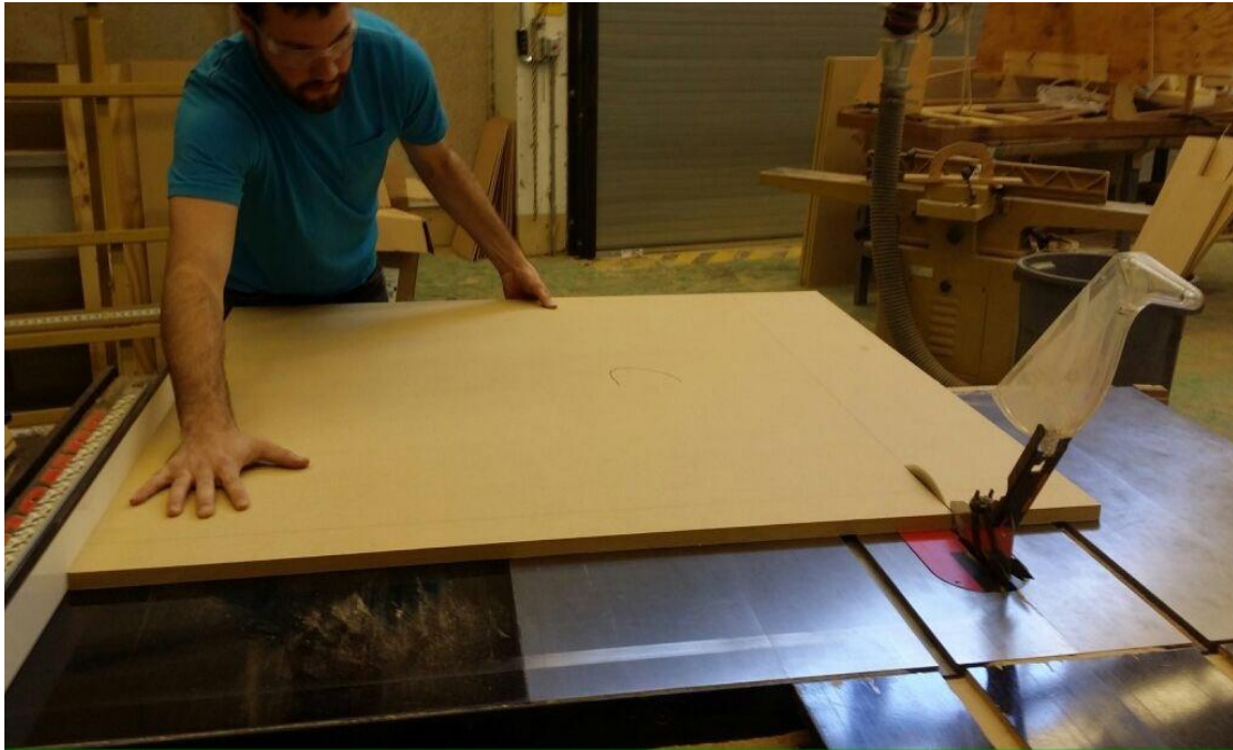
Figure 18. One of the panels is trimmed using the table saw
