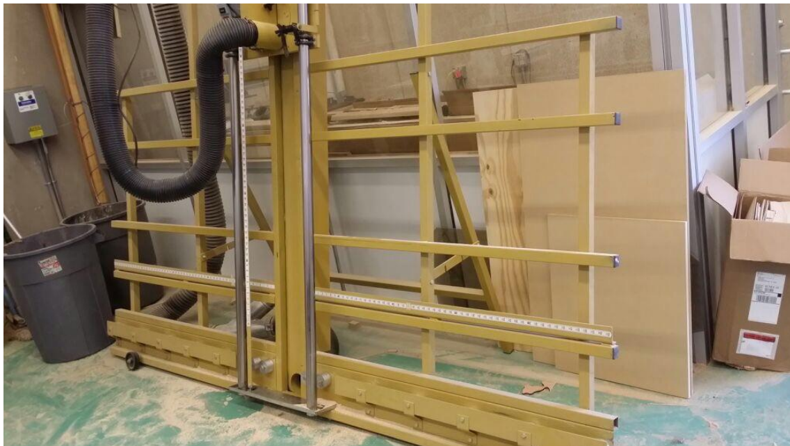
Figure 17. Panel saw used to cut the panels
