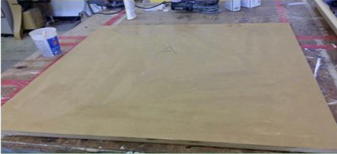
Figure 21. Panel A coated with a mixture of epoxy and denatured alcohol
