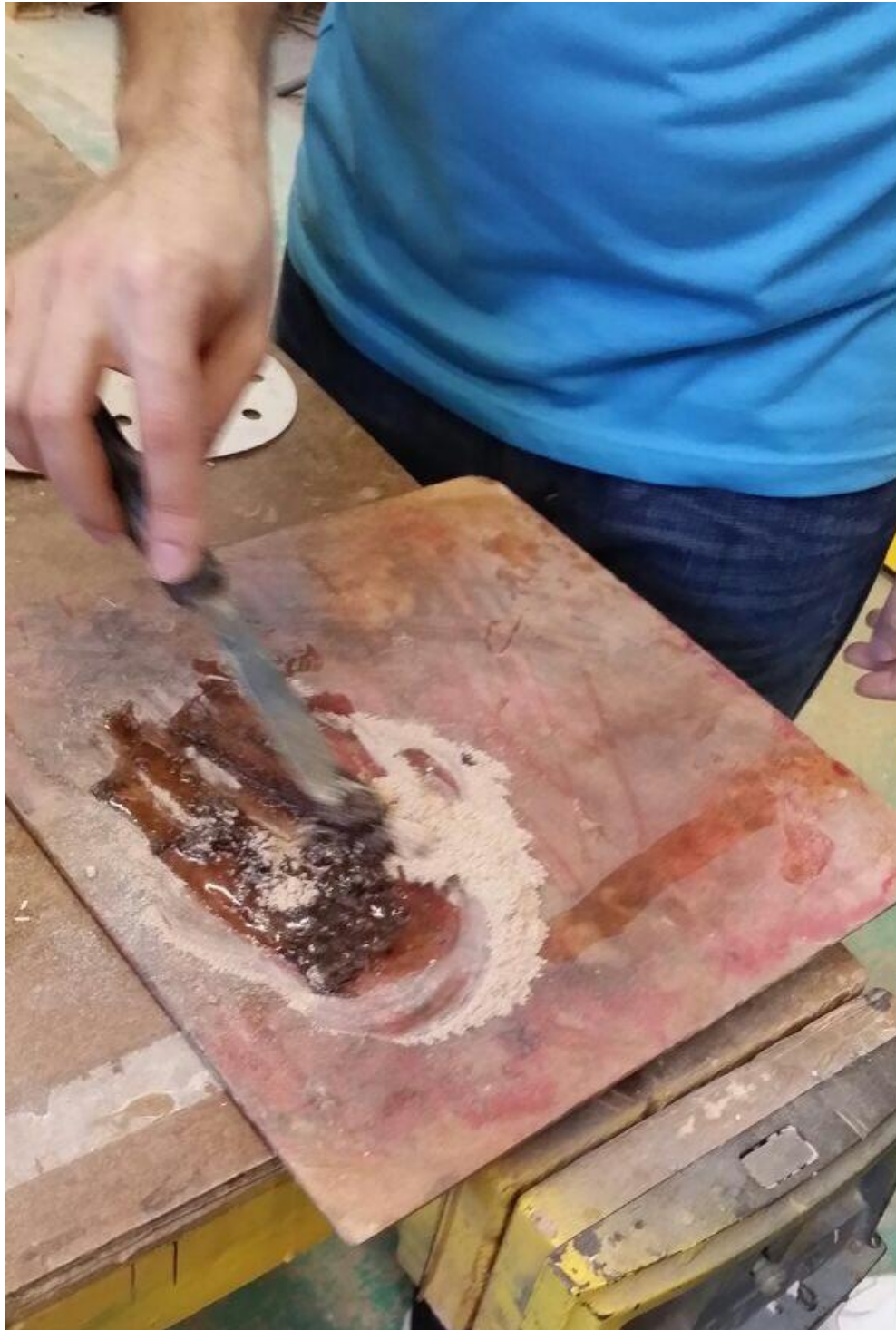
Figure 23. Epoxy and wood dust being mixed
