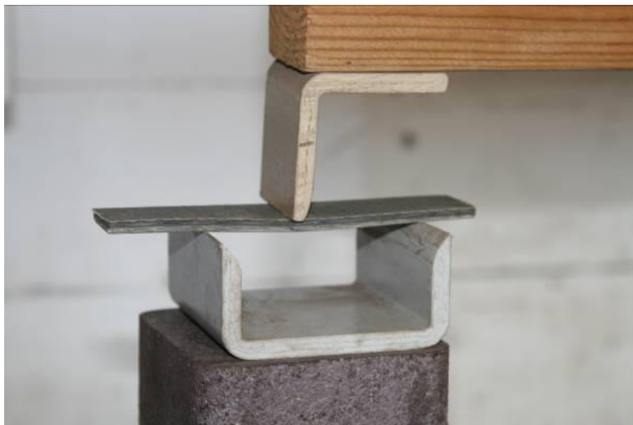
Figure 10.22. Breaking a coupon of carbon fiber and fiberglass composition to test the flexural breaking strength of the laminate stack. Photo courtesy Conservation Research Lab and the Texas Historical Commission.
