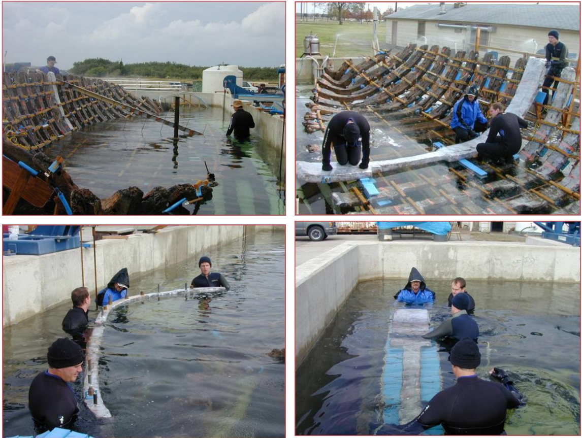
Figure 10.25. Upper left, Hitchcock and Pevny setting the gauge for jig. Upper right, reconstruction team in the process of wrapping the midship frame with cellophane plastic. Lower left, the team using buoyancy to help move the framesets to the jig. Lower right, the midship frame sitting on the jig awaiting the casting sequence. Photo courtesy Conservation Research Laboratory and the Texas Historical Commission.
