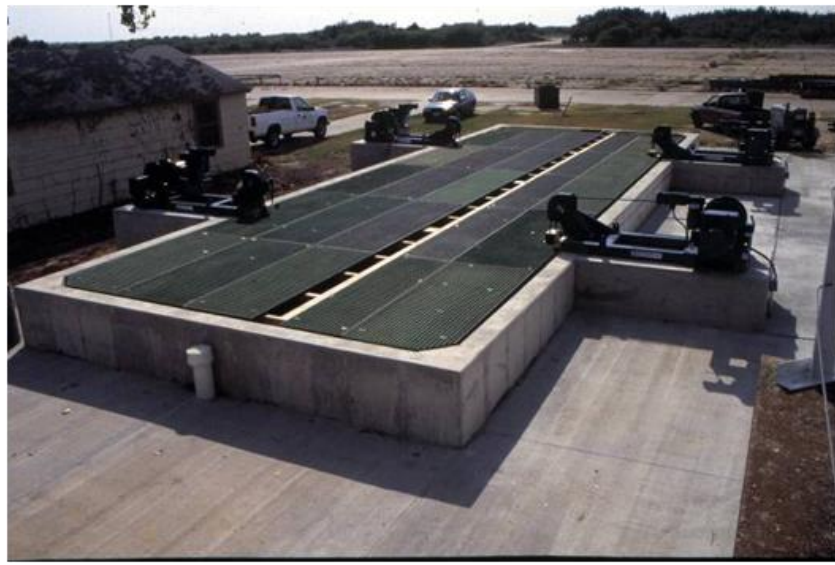
Figure 10.14. The Conservation Research Lab, ship conservation vat at Texas A&M University. The deck, controlled by four synchro-winches cantilever from the side allows for easy access. Note the gap offset to the right of center (as viewed). The gap delineates the centerline footprint for the boat. Photo courtesy Texas A&M Conservation Research Laboratory and the Texas Historical Commission.
