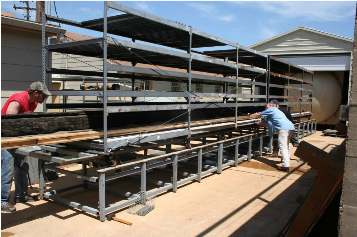
Figure 10.30. CRL staff loading the keel and its base onto the freeze-drying rack system. In order to ensure that the irregular surface on the underside of the keel remained consistent during the drying process the fiberglass plate was left attached to the timber. Photograph courtesy Conservation Research Laboratory and the Texas Historical Commission.
