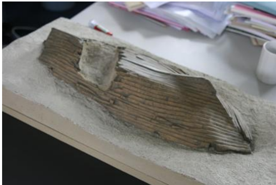
Figure 6.3. A "printed" solid model of the up-turned Doel Kogge 1 produced by data from the three-dimensional scan of the cog as found. Note the sediments propping up the hull through the 4 m gash created by the bucket of mechanical excavator. Photograph from the author's personal collection.
