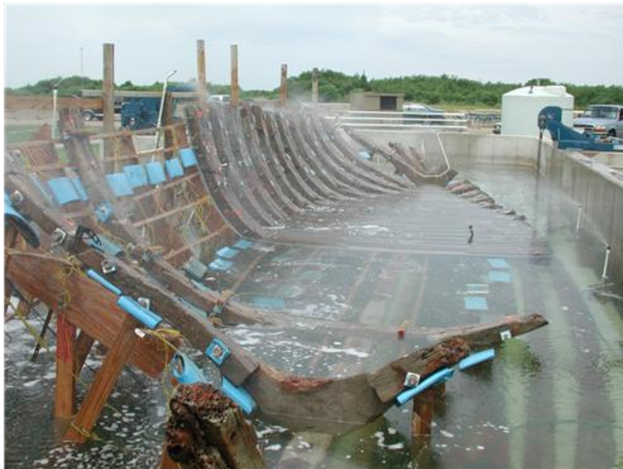
Figure 10.21. Looking aft and across the hull to starboard. The line of rectangular pads marks the location of poppet runs. Between the puppets on starboard the external basket created by rows of buttons is visible with the framesets removed. The hull is being misted with water. Photo courtesy Conservation Research Laboratory and the Texas Historical Commission.
