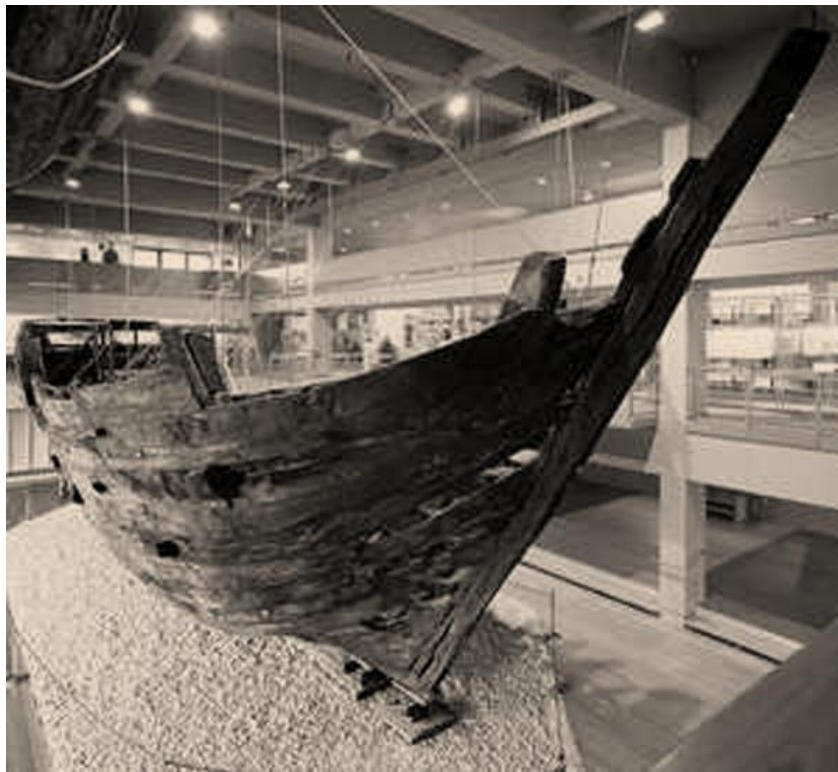
Figure 9.3. The Bremen Cog support system. Photograph from the author's personal collection—video capture.
