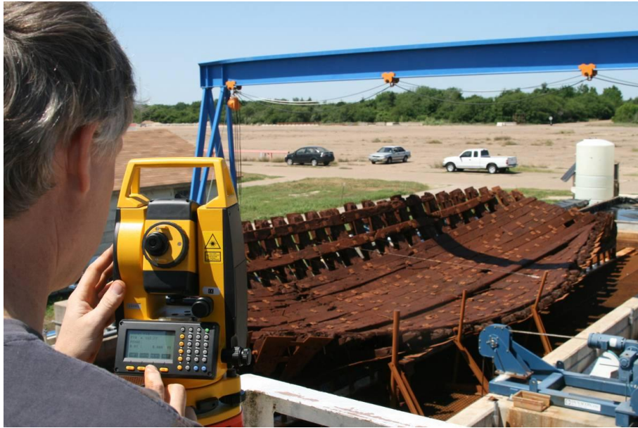
Figure 10.28. Using a total station to pick point the ceiling runs of La Belle before disassembly. Photograph courtesy Conservation Research Laboratory
