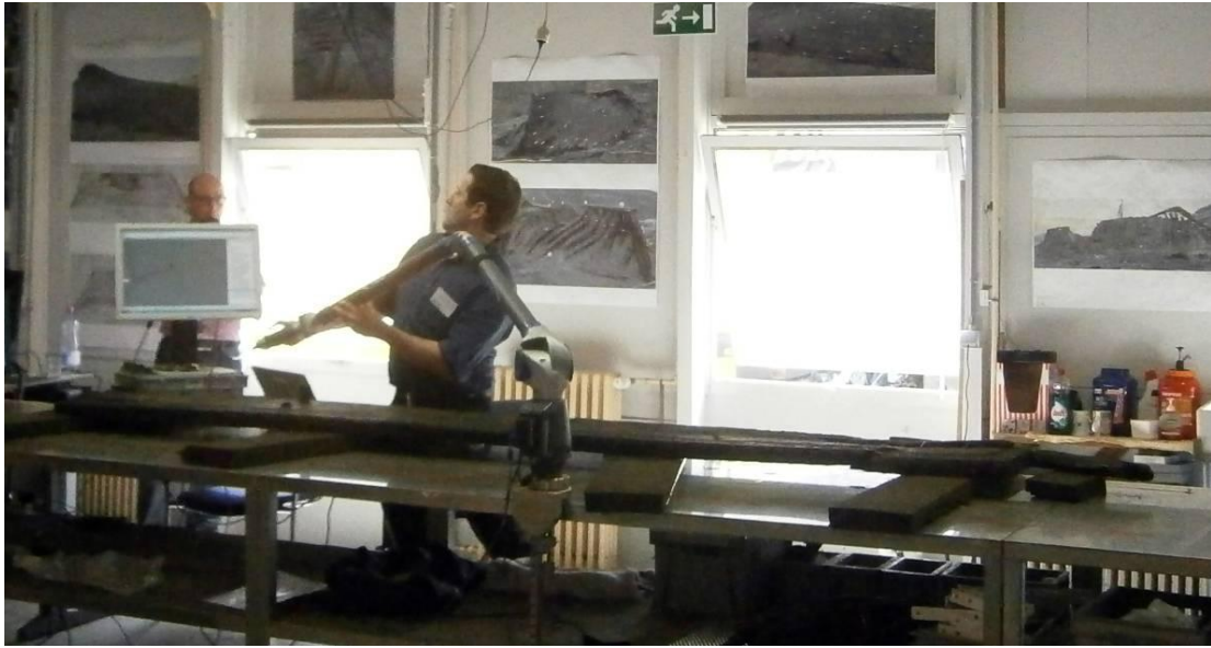
Figure 5.6. Using a Faro Arm® to record a plank from the Doel Kogge. Photograph from the author's personal collection.
