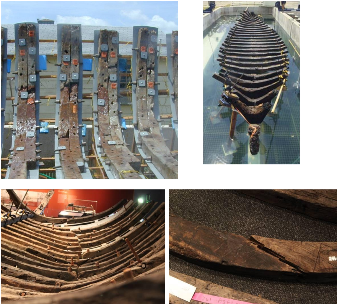
Figure 10.6. Clockwise from top left. Frame sets “D-1” through “D-4” starboard, illustrating the formation of the frames by joining overlapping futtocks. Upper right, looking aft at the symmetry formed in the floor length by the narrowing lines and the natural breaking point the lengths create. Lower left, the longitudinal seam created in the hull construction by not staggering the length of the floors and second futtocks. The longitudinal break placed considerable strain on the first futtocks. Lower right, an example of the first futtocks cross-grain fracture. Photograph courtesy Texas A&M University Conservation Research Laboratory and The Texas Historical Commission.
