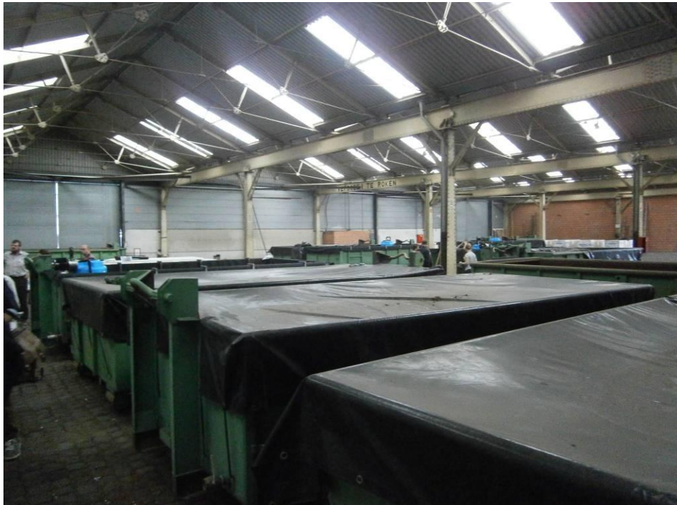
Figure 7.2 The rows of vats that will be used to saturate the timbers of the Doel Kogge with PEG. Photograph from the author's personal collection.
