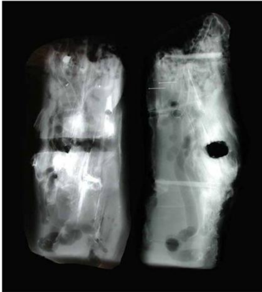
Figure 10.8. An x-ray of a degraded third futtock from La Belle approximately 18 inches long illustrating the depth and extent of shipworm penetration. X-ray courtesy Conservation Research Laboratory.
