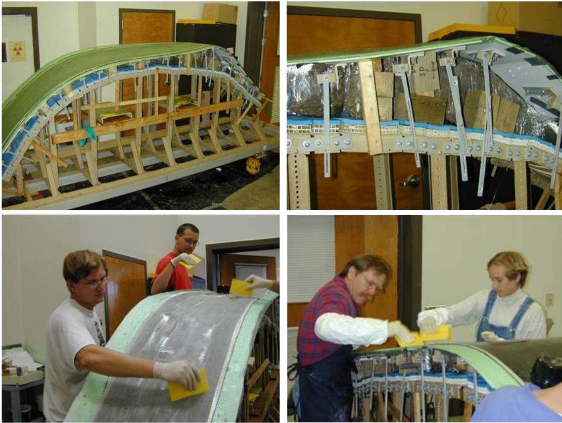
Figure 10.26. Upper left, the jig with frame set in the process of vacuum bagging the stack. Upper right, the manner in which wings were attached along the side of the framesets in order to create an edge that extended beyond the actual frame. Lower and right, conservation research lab staff and guest work epoxy into the laminate stack the casting sequence. Photo courtesy Conservation Research Laboratory and the Texas Historical Commission.
