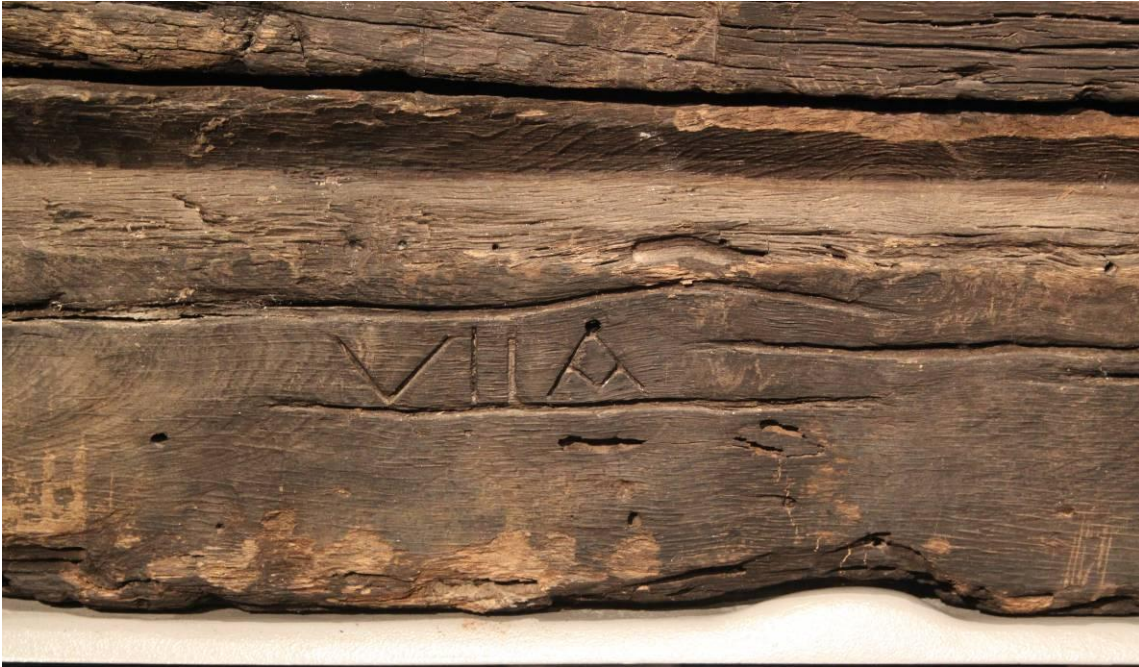
Figure 10.2. Since the hull was originally to be constructed en fagot , the inscribed mark “VII A” designates the correct orientation of the floor at this point on the keel, which is seven frame sets forward of the master frame. Photograph courtesy, The Texas A&M University Conservation Research Lab and The Texas Historical Commission.
