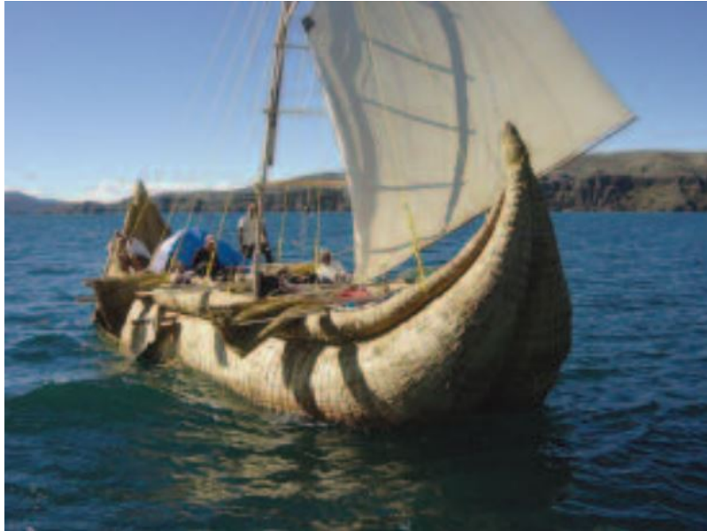
Figure 3.9: The experimental totora reed boat sailing on Lake Titicaca. Note the bipod mast and upturned ends (from Vranich et al. 2005, 24).
