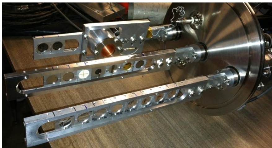
Figure 2.1. Target ladder flange assembly for use with the MARS primary target chamber. Shown front to back: degrader ladder with Al degraders, target ladder with target foils and fluorescent (ZnCdS) viewer, and carbon foil ladder with an electron-suppressed Faraday-cup and two ^{nat}\text{C} foils.
