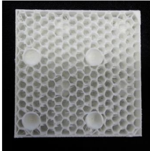
Figure 5.1 Porosity of the printed PLA with 10% infill
