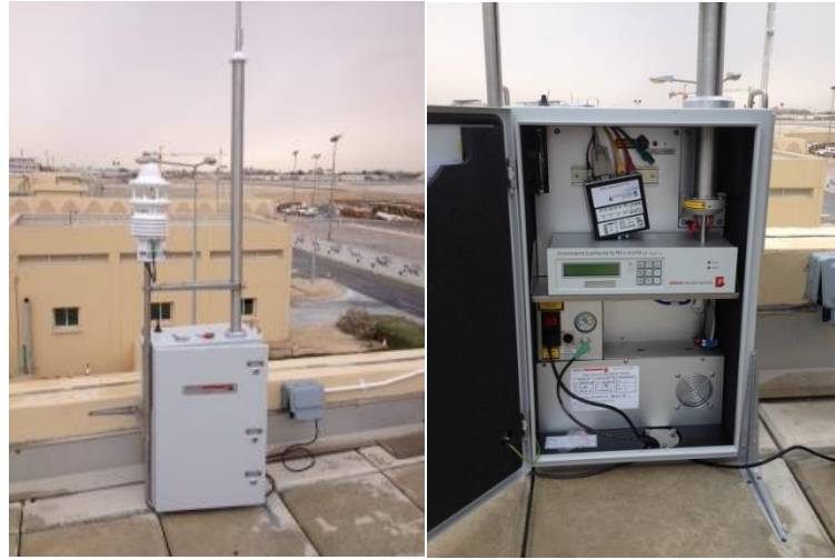
Figure 2 Environ Check 365# air quality monitoring station (by Grimm Aerosol Technik GmbH & Co. KG, Germany)
