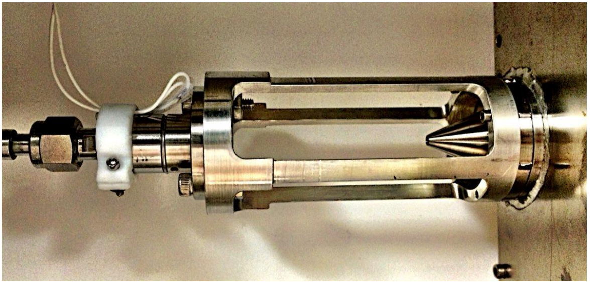
Figure 3 - 11: Stationary Valve - Testing
